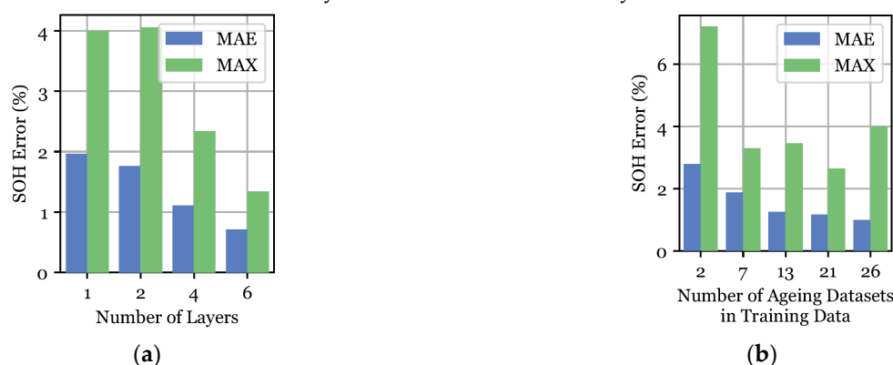
Figure 5. (a) Estimation accuracy over validation data versus number of layers in CNN. (b) Estimation accuracy measured during validation versus number of training datasets. All tests were performed over validation datasets recorded at 25 °C.
