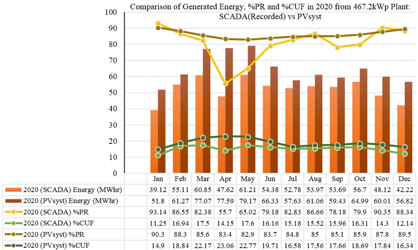
Figure 10. Comparison of Generated Energy, %PR and %CUF in 2020 from 467.2 kWp Plant: SCADA (Recorded) vs. PVsyst.
