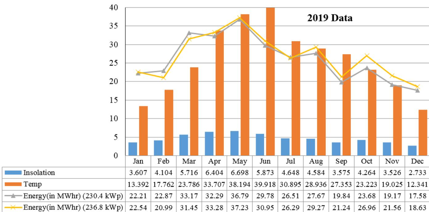
**Figure 6.** Comparison of Generated Energy in 2019 (P<sub>1</sub> vs. P<sub>2</sub> + P<sub>3</sub>).
