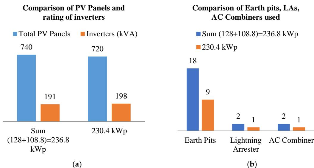
**Figure 4.** (a) Comparison of required rating of inverters, SPV panels in Plant ‘P<sub>2</sub> + P<sub>3</sub>’ and Plant ‘P<sub>1</sub>’. (b) Comparison of required Earth Pits, Lightning Arresters, AC Boxes in Plant ‘P<sub>2</sub> + P<sub>3</sub>’ and Plant ‘P<sub>1</sub>’.
