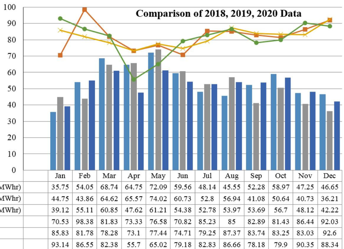
**Figure 8.** Comparison of Generated Energy in 2018, 2019, and 2020 of 467.2 kWp Plant ( $P_1 + P_2 + P_3$ ).
