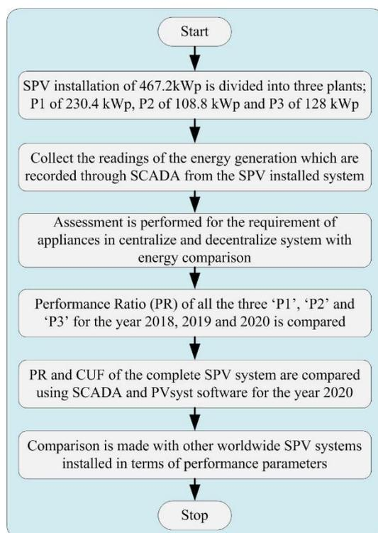
Figure 1. Methodology followed for assessment and comparison of SPV plant.
