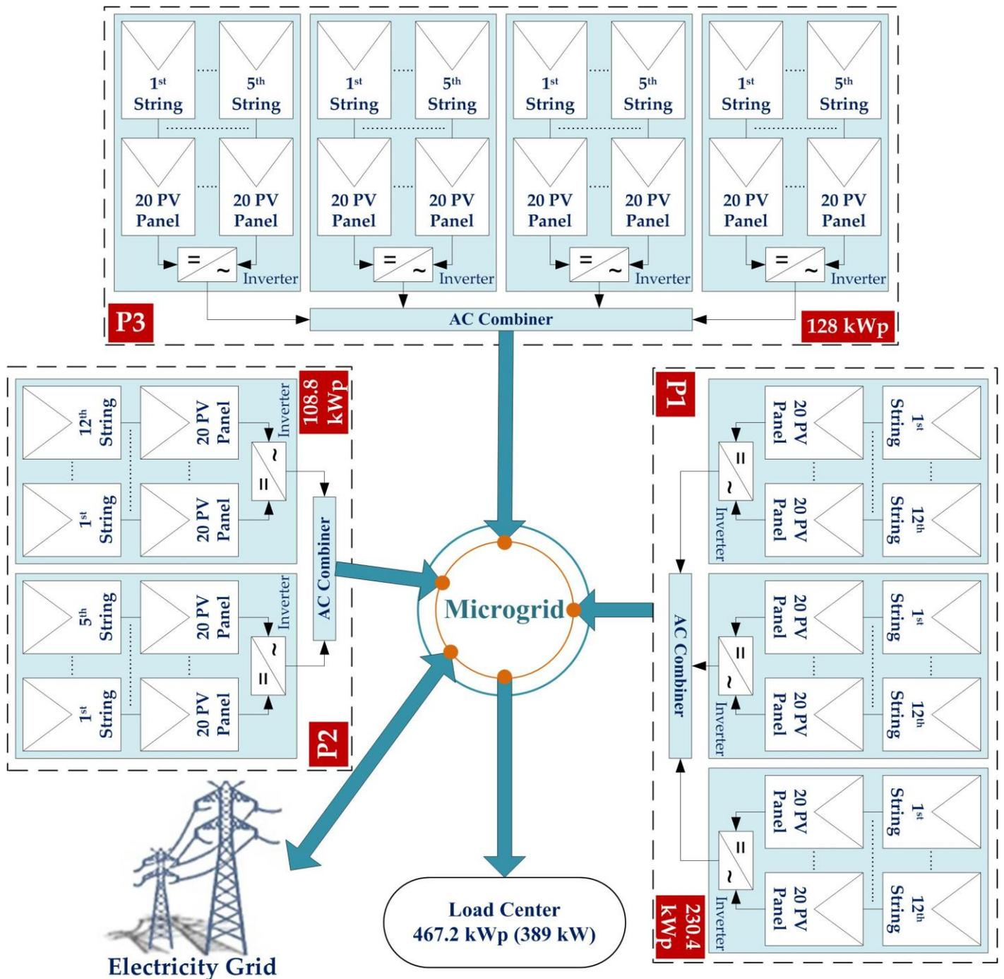
Figure 2. Developed electrical microgrid scheme based on solar PV system (1460 no. of PV panels (320 Wp) = 467.2 kWp (389 kW)).
