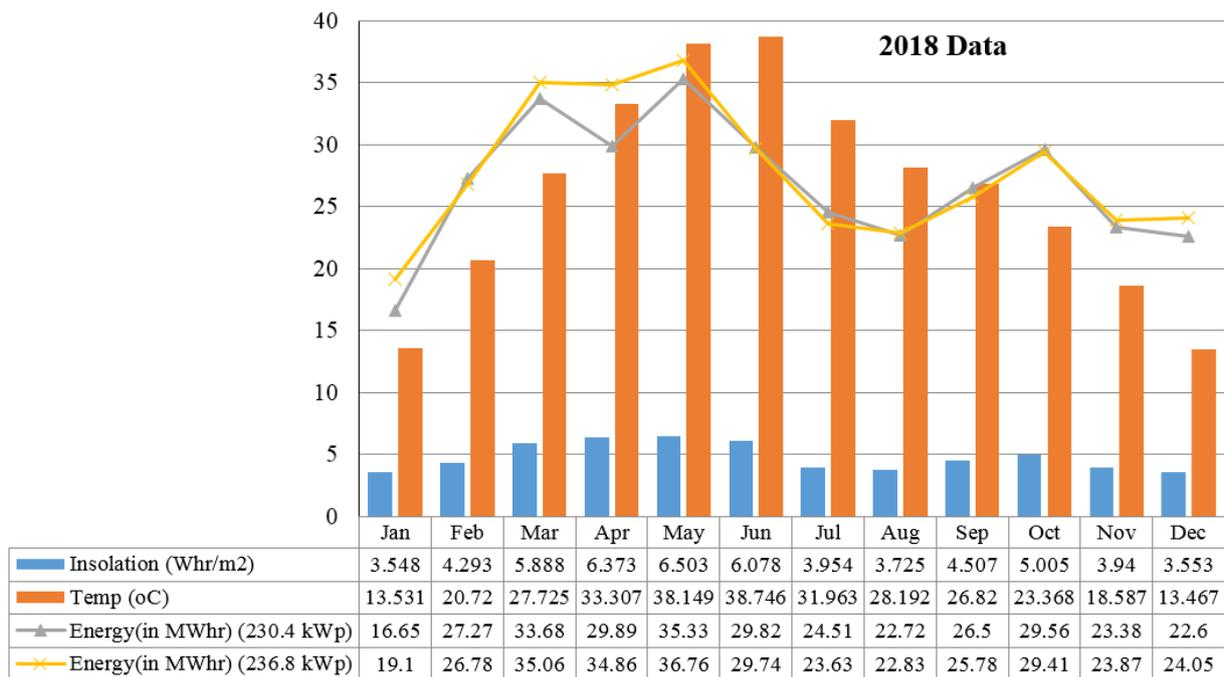
**Figure 5.** Comparison of Generated Energy in 2018 (P<sub>1</sub> vs. P<sub>2</sub> + P<sub>3</sub>).
