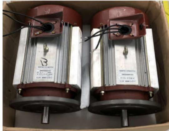
**Figure 16.** The manufactured LSPMSM.
