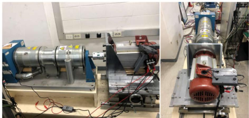
**Figure 17.** Test setup of the LSPMSM.
