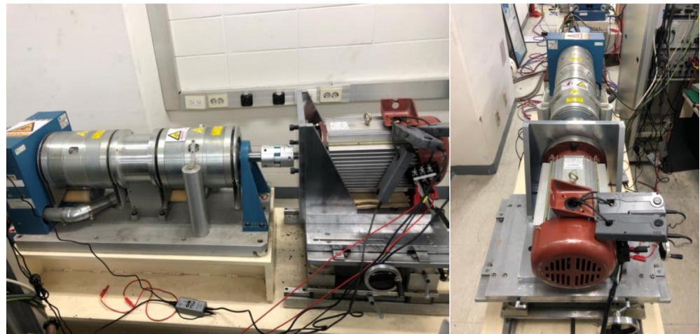
Figure 17. Test setup of the LSPMSM.
