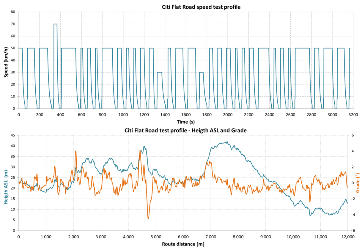
Figure 9. City Flat Road test profile (speed, absolute altitude, and grade).
