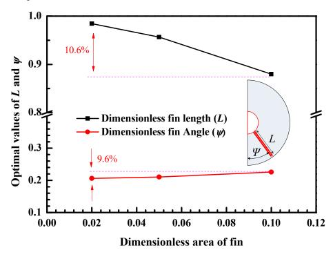
**Figure 12.** Variation of the optimal dimensionless fin length, *L*, and dimensionless fin angle,  $\psi$ , with the dimensionless fin area, *A*.
