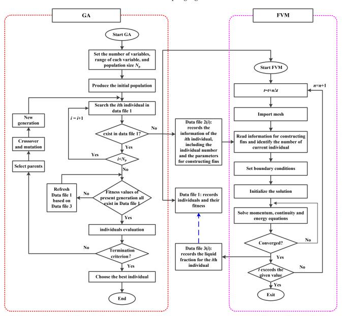
Figure 4. The flowchart of the optimization process.
