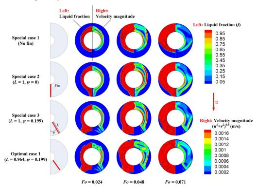
**Figure 7.** Contour maps of liquid fraction and velocity magnitude for Special Cases 1–3 and Optimal Case 1.
