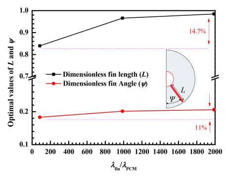
**Figure 9.** Variation of the optimal dimensionless fin length, *L*, and dimensionless fin angle,  $\psi$ , with the thermal conductivity ratio of fin to PCM ( $\lambda_{\text{fin}}/\lambda_{\text{PCM}}$ ).
