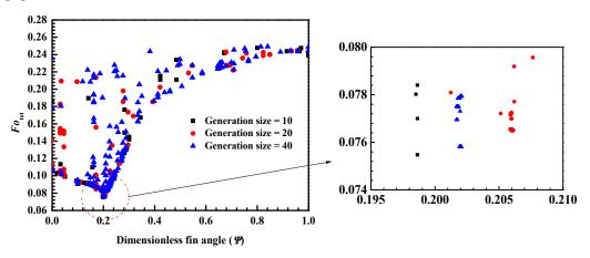
**Figure 6.** Different dimensionless fin angles generated by genetic algorithm (GA) with different population sizes.
