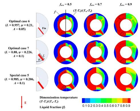
have almost the same melting process, and the PCM in the upper and lower region of the fin has a similar melting ratio.
