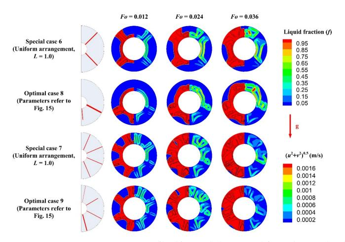
**Figure 16.** Contour maps of liquid fraction and velocity magnitude for Special Cases 6 and 7 and Optimal Cases 8 and 9.
