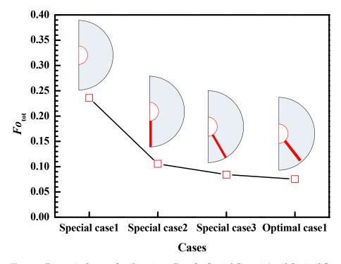
Figure 8. Dimensionless total melting time, Fotot, for Special Cases 1–3 and Optimal Case 1.
