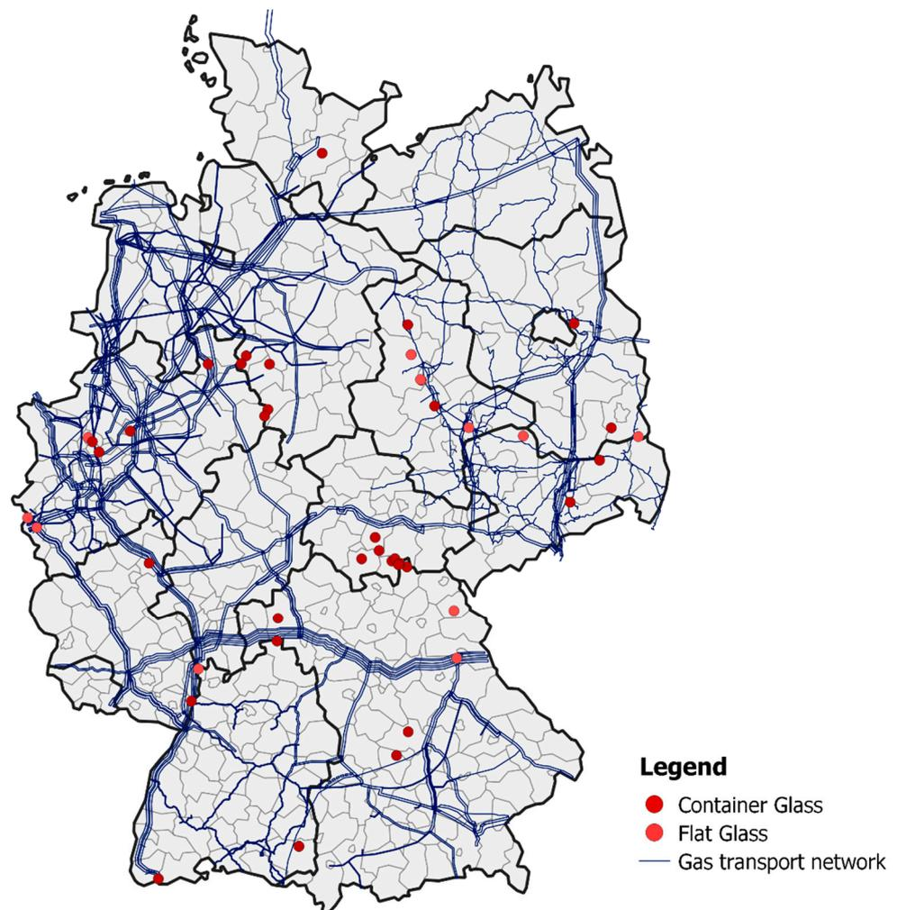
**Figure 6.** Glass production sites in combination with the current gas transportation network. Dark red circles are production sites for container glass and light red circles are production sites for flat glass. Based on [26,34] and updated from [27].
