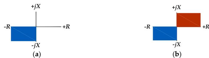
**Figure 4.** Fault discrimination characteristics: (a) internal faults; (b) external faults.
