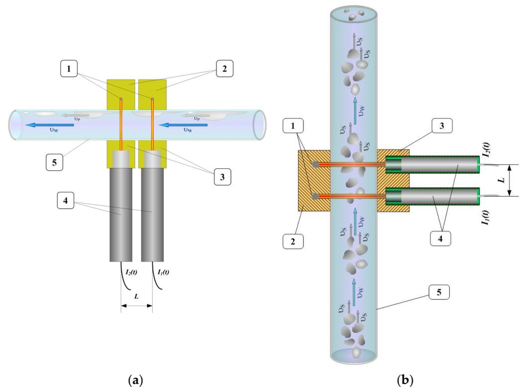
**Figure 1.** Basic schema of measurement of gamma absorption of the following flows: (a) gas–liquid flow in a horizontal pipeline and (b) solid particles transported by a liquid in a vertical pipe; 1—sealed gamma-ray sources; 2—lead collimator of the source; 3—lead collimator of the scintillation probes; 4—scintillation probes; 5—pipeline.
