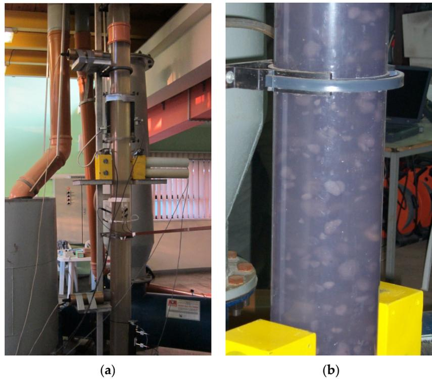
**Figure 4.** Fragments of the installation for testing liquid–solid particles flow in a vertical pipe: (a) view of the measuring part of the laboratory stand; (b) pipe with the water–solids mixture [36].
