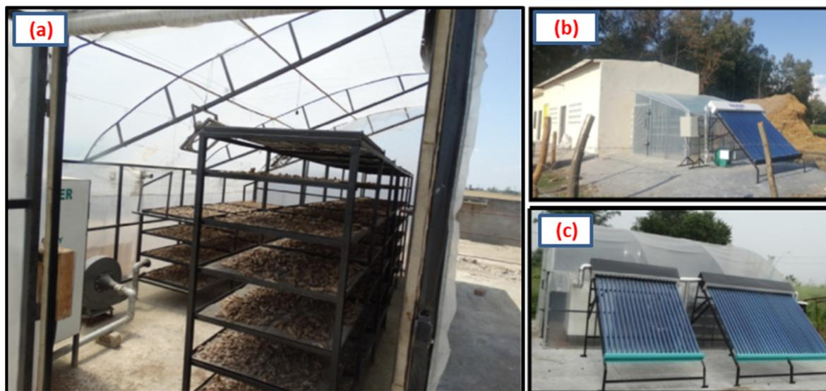
**Figure 6.** (a) Drying arrangement inside a greenhouse and (b,c) photos of a few installations [96], with permission No. 5413090348588.
