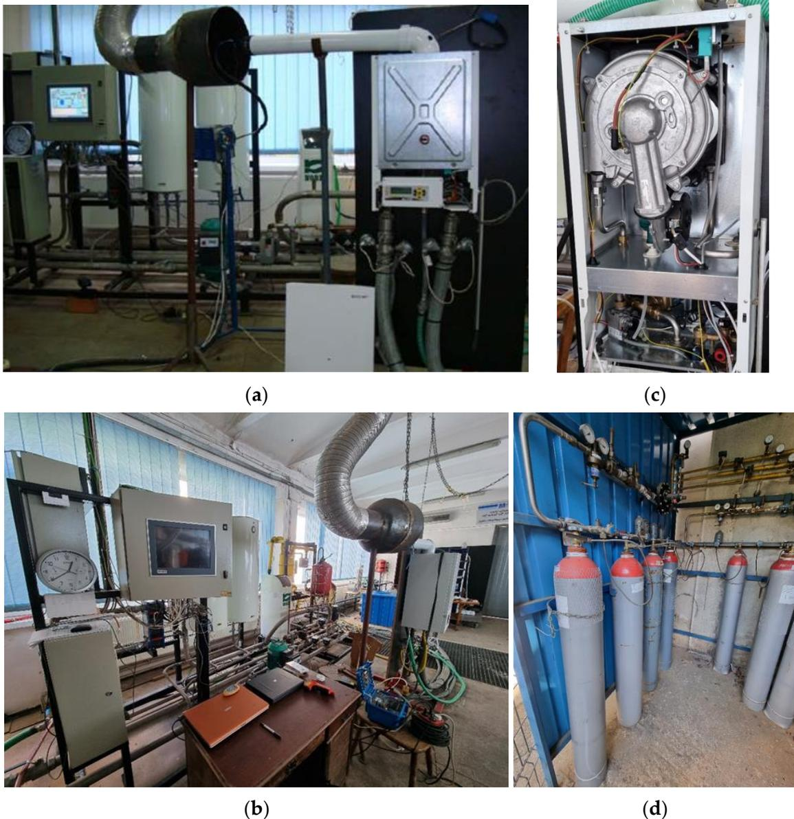
**Figure 1.** (a,b) Experimental stand; (c) Flattened pipes boiler, and (d) Gas supply plant.
