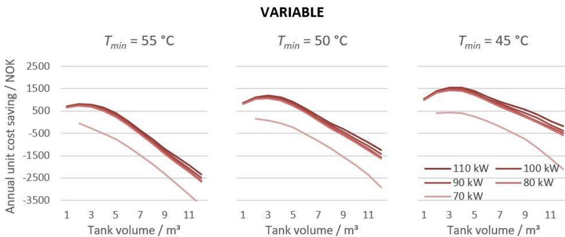
**Figure 13.** Unit cost saving as a function of the tank volume for variable setpoint demand profile at different maximum heating power and minimum tank temperature using 2019 spot prices. 1 NOK  $\approx$  0.1 EUR.
