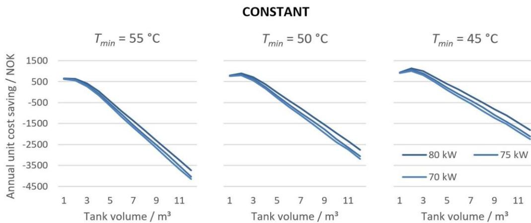
**Figure 14.** Unit cost saving as a function of the tank volume for constant setpoint demand profile at different maximum heating power and minimum tank temperature using 2019 spot prices. 1 NOK  $\approx$  0.1 EUR.
