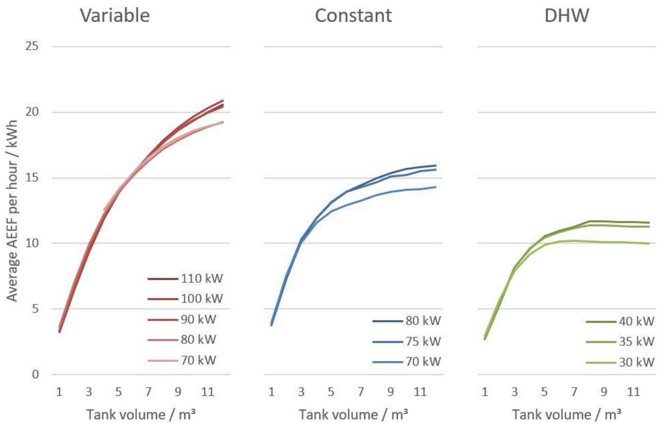
**Figure 11.** Average AEEF per hour as a function of tank volume for the three demand profiles at different maximum heating power using 2019 spot prices.
