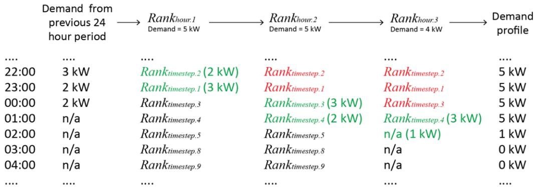
**Figure 7.** Graphical representation of demand profile optimisation for a simple example of a heating element with a 5 kW capacity. Green shows placement of an hour’s demand at that timestep. Red shows where demand placement is not possible as the capacity of that timestep has already been reached.
