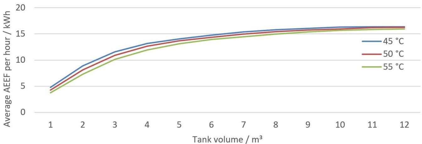
**Figure 12.** Effect of minimum setpoint temperature on AEEF as a function of tank volume. Result for constant setpoint heating and 80 kW heating power using 2019 spot prices.
