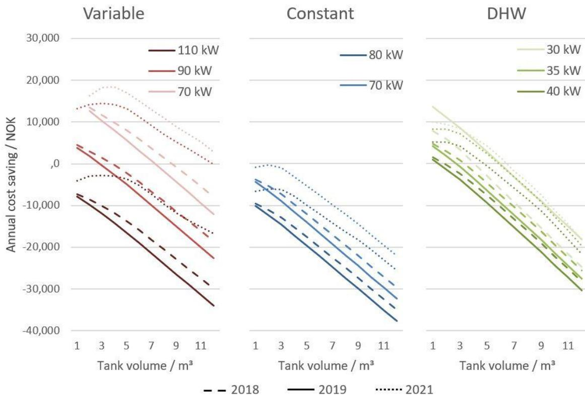
**Figure 19.** Total annual cost saving as a function of the tank volume for the three demand profiles at different maximum heating power using 2018, 2019 and 2021 spot prices. 1 NOK  $\approx$  0.1 EUR.
