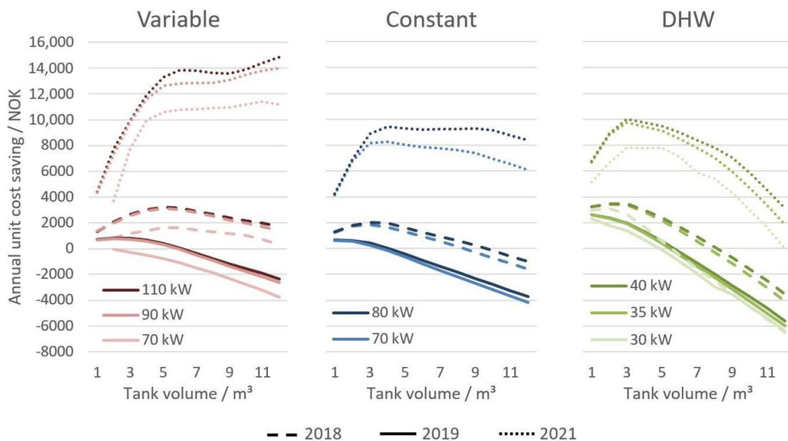
**Figure 17.** Unit cost saving as a function of the tank volume for the three demand profiles at different maximum heating power using 2018, 2019 and 2021 spot prices. 1 NOK ≈ 0.1 EUR.
