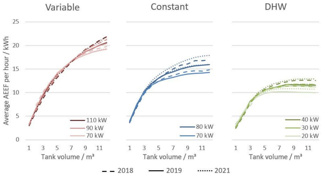
**Figure 16.** Average AEEF per hour as a function of tank volume for the three demand profiles at different maximum heating power using 2018, 2019 and 2021 spot prices.
