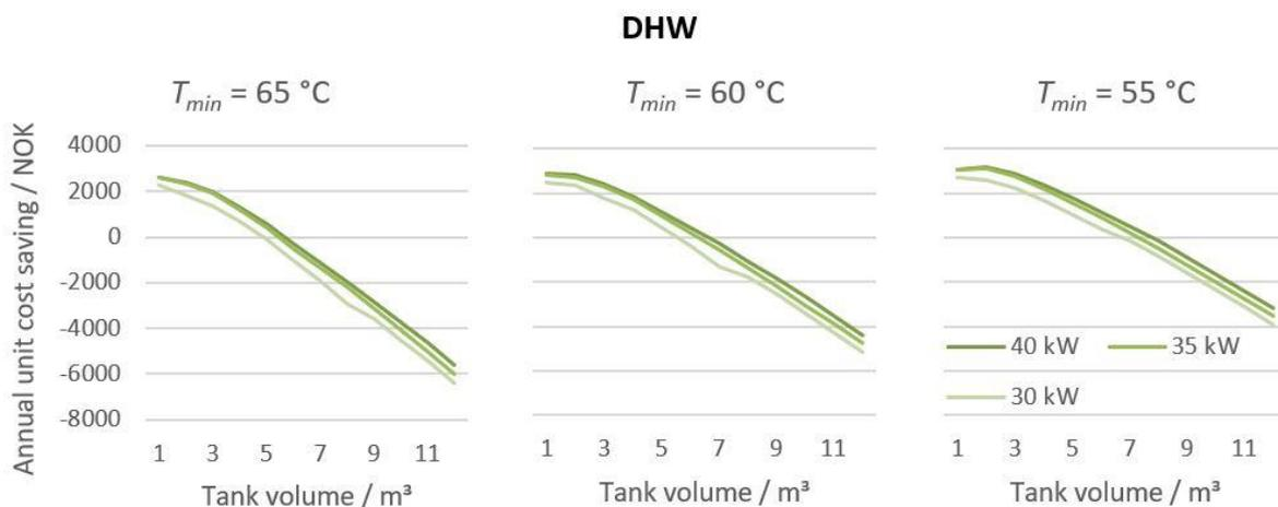
**Figure 15.** Unit cost saving as a function of the tank volume for DHW demand profile at different maximum heating power and minimum tank temperature using 2019 spot prices. 1 NOK  $\approx$  0.1 EUR.
