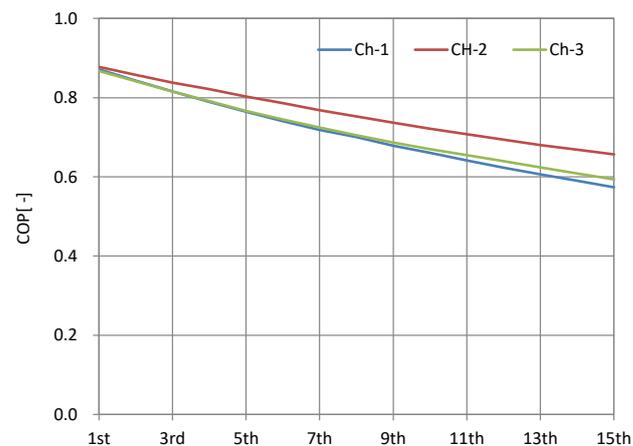
**Figure 9.** Annual average COP change for heat source equipment.
