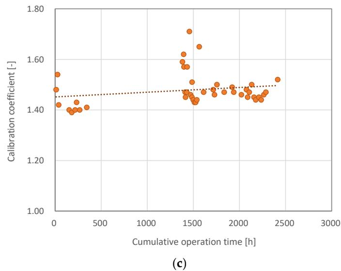
**Figure 4.** Calibration coefficient values according to the cumulative operation time of the pumps: (a) P-1; (b) P-2; (c) P-3.
