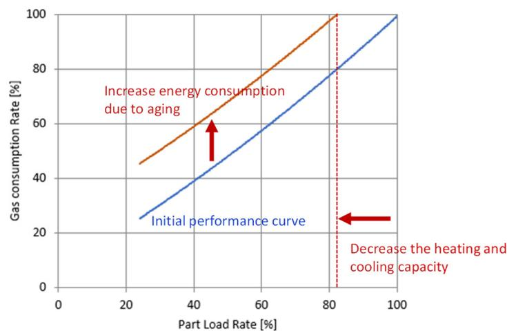
Figure 6. Concept of performance degradation of heat source equipment.
