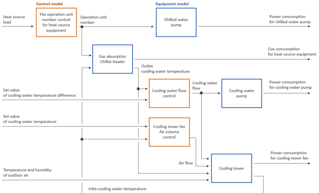
Figure 5. Simulation flow chart.
