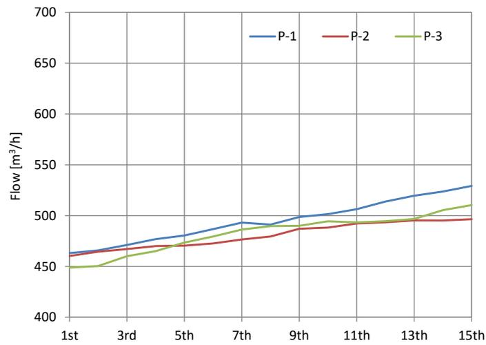
Figure 12. Average annual change in flow rate for cooling water pumps.
