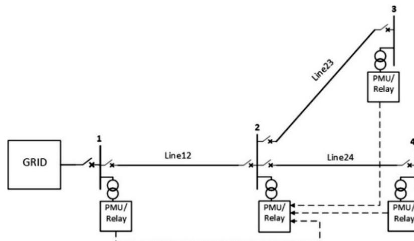
Figure 2. Application of a new type of voltage relays based on PMU [69].
