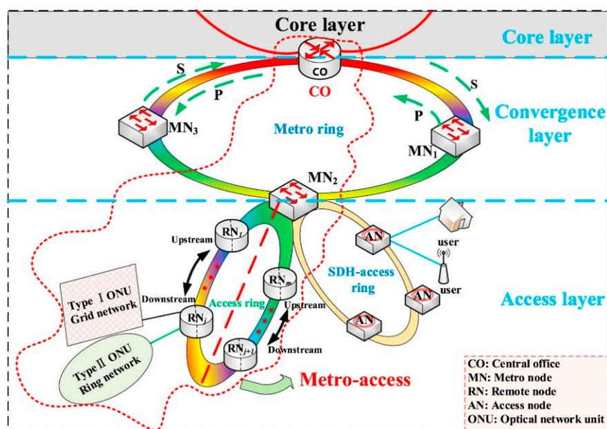
**Figure 3.** Diagram of network architecture of differential protection with optical fiber communication lines [58].
