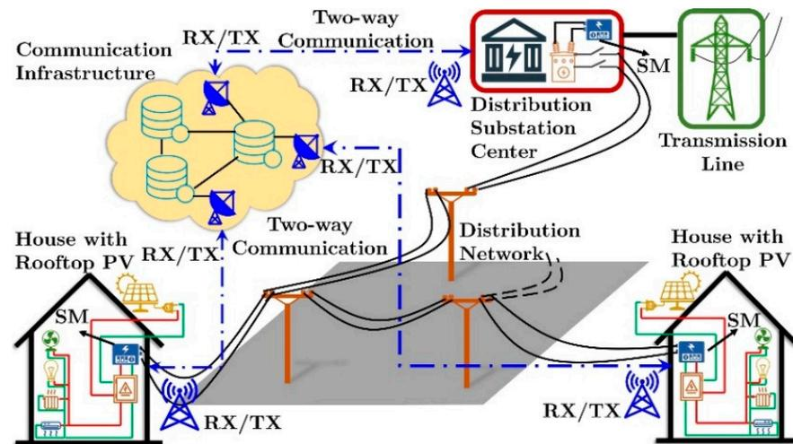
Figure 1. Effective use of smart meters in microgrids with DERs [65].
