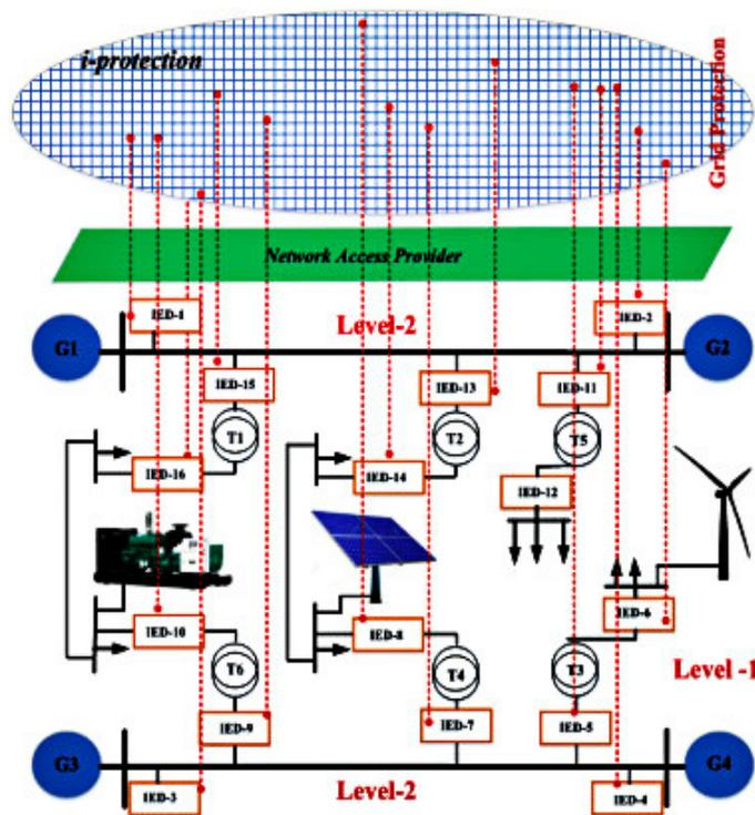
Figure 5. New relay topology based on *i*-protection [105].
