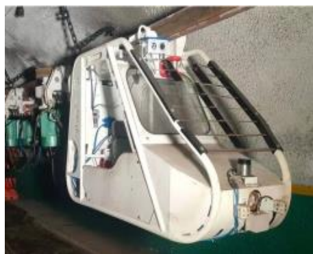
Figure 15. Xinsha monorail equipment monorail crane.
