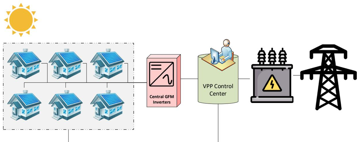
Figure 5. Schematic of a grid-forming VPP without energy storage.
