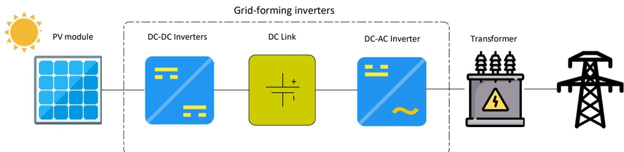
Figure 4. Schematic of grid-forming inverters.
