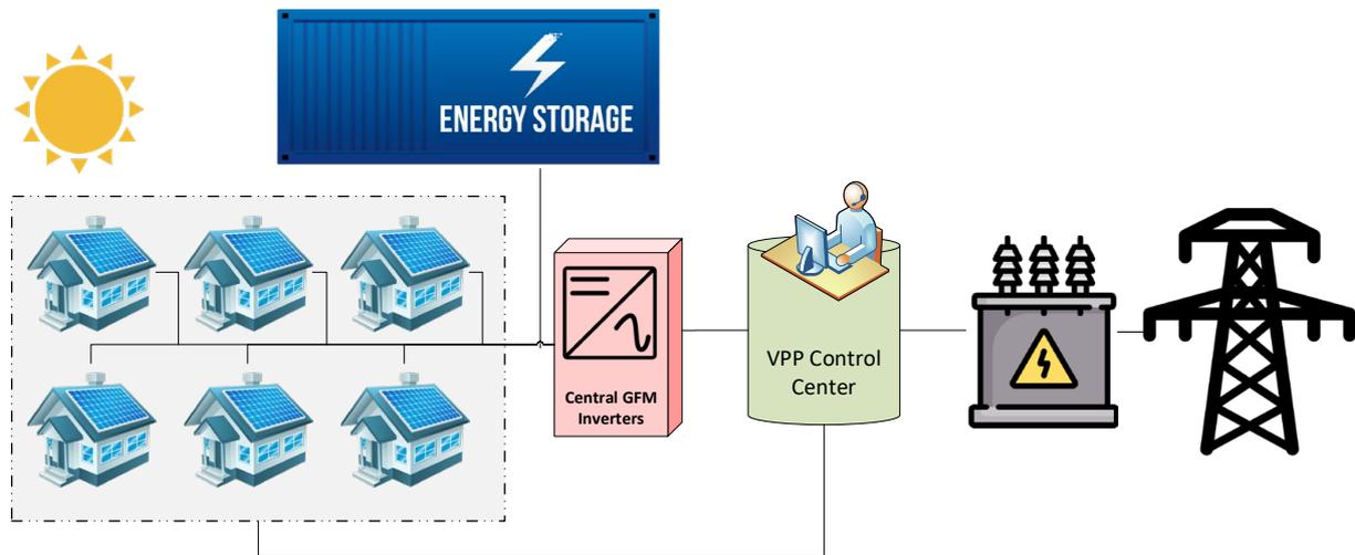
**Figure 6.** Schematic of a grid-forming VPP with energy storage.
