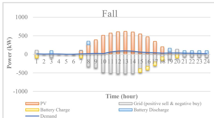
Figure 12. The bidding power of the VPP in fall.
