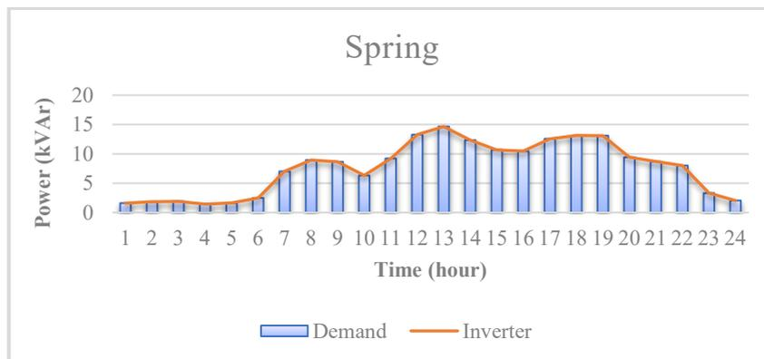
Figure 17. The reactive power support by smart inverters in spring.
