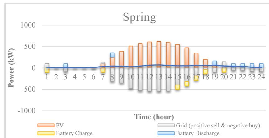
Figure 16. The bidding power of the VPP in spring.
