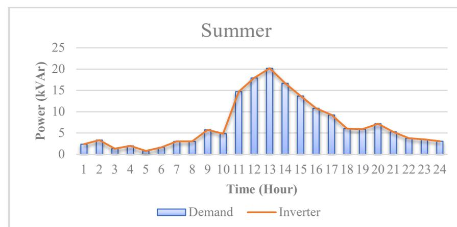
**Figure 11.** The reactive power support by smart inverters in summer.
