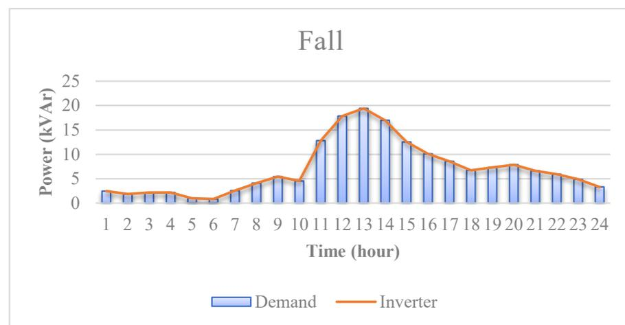
Figure 13. The reactive power support by smart inverters in fall.
