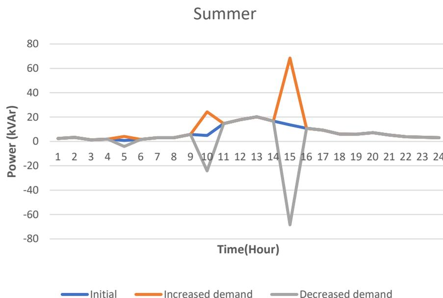
**Figure 19.** The reactive power provided by smart inverters in summer when demand varies.
