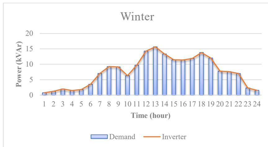
Figure 15. The reactive power support by smart inverters in winter.
