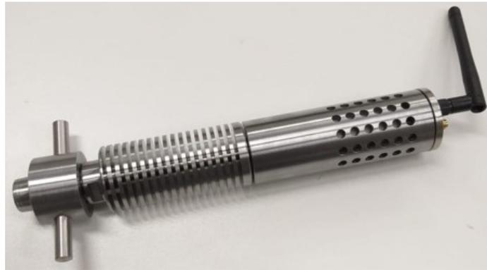
**Figure 3.** In-cylinder pressure sensor developed in Ref. [21].
