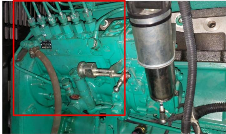
**Figure 8.** Injection pump at the ICE.
