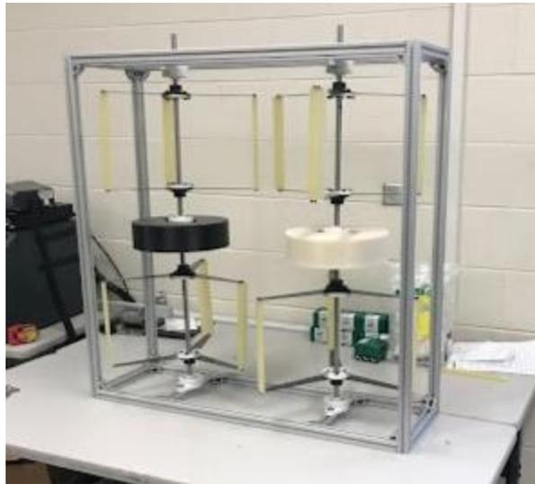
**Figure 4.** Photograph of the assembled DD-VADHT scaled prototype.
