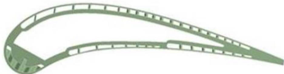
Figure 29. Example of F-type first nozzle cooling design concept of 3D printed internal cooling design [85].
