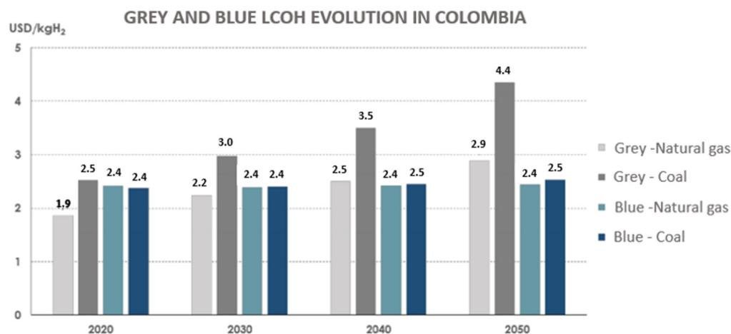
**Figure 10.** LCOH of coal and natural gas for blue and grey H<sub>2</sub> production [3].
