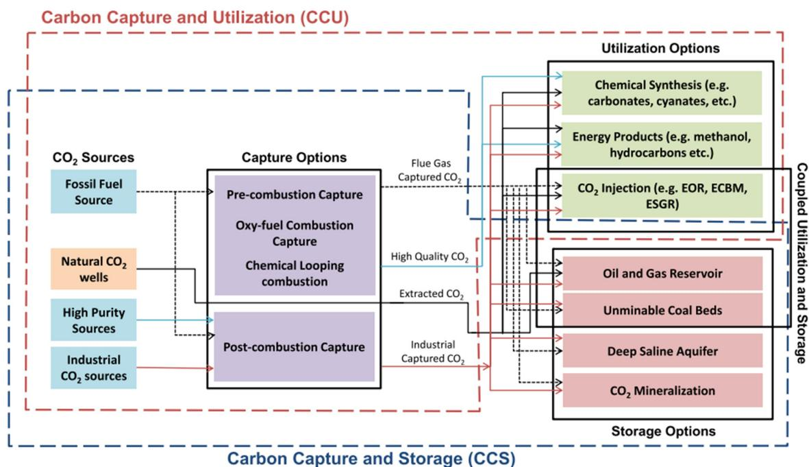
**Figure 8.** CCUS structure with different storage and utilization paths [34]. Reprinted with permission from Elsevier.
