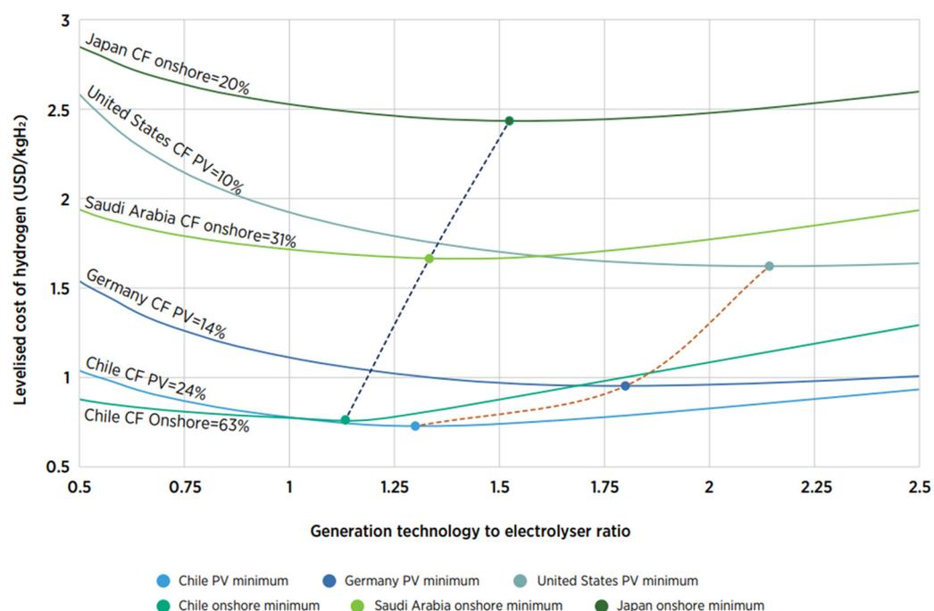
**Figure 5.** LCOH produced by different means vs. generation technology ratio and CF for NZE scenario [19].
