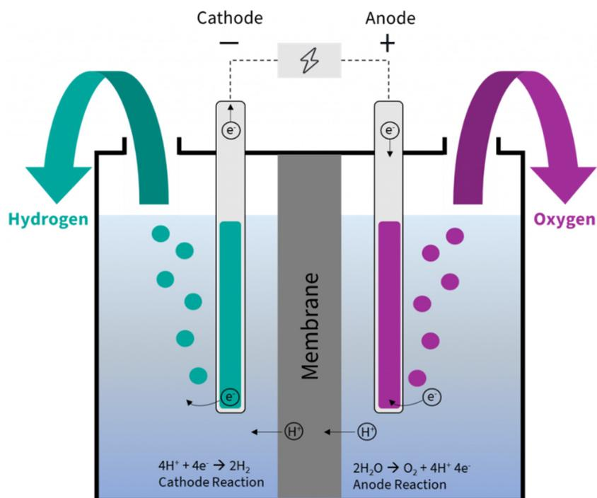
**Figure 4.** Simplified scheme of the water electrolysis process [21].
