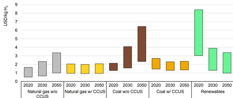
**Figure 6.** Comparison of hydrogen production costs with different technologies and scenarios [2].
