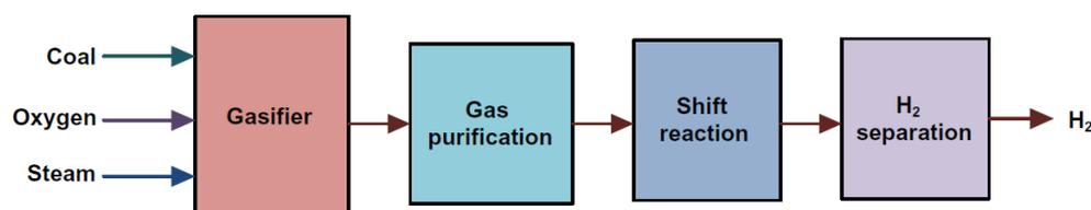
**Figure 2.** Hydrogen production by the coal gasification process [8]. Reprinted with permission from Elsevier.
