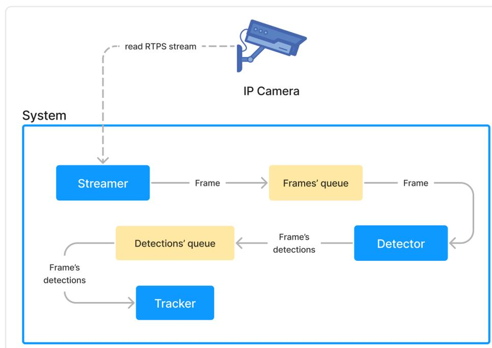
**Figure 1.** Diagram of the system architecture, showing the three main modules and data queues.
