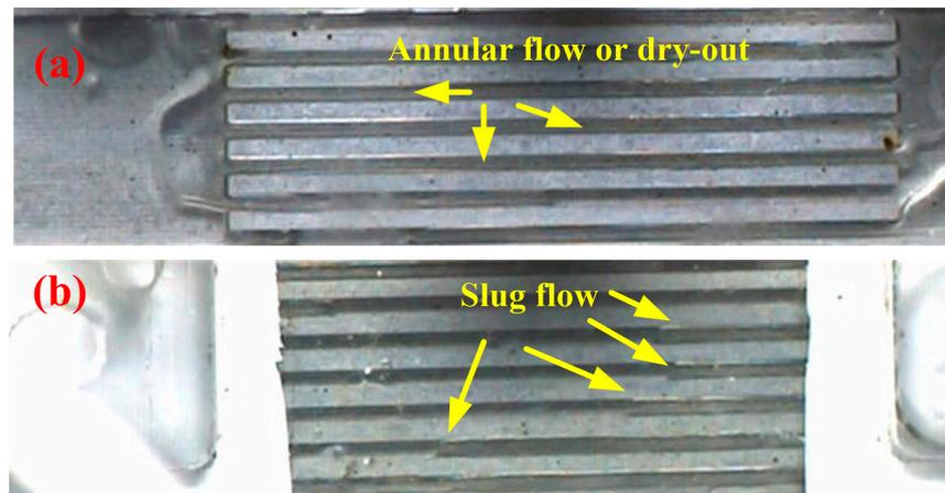
**Figure 12.** Effect of vapor venting membrane on the flow regime: (a) Without membrane; (b) With membrane.
