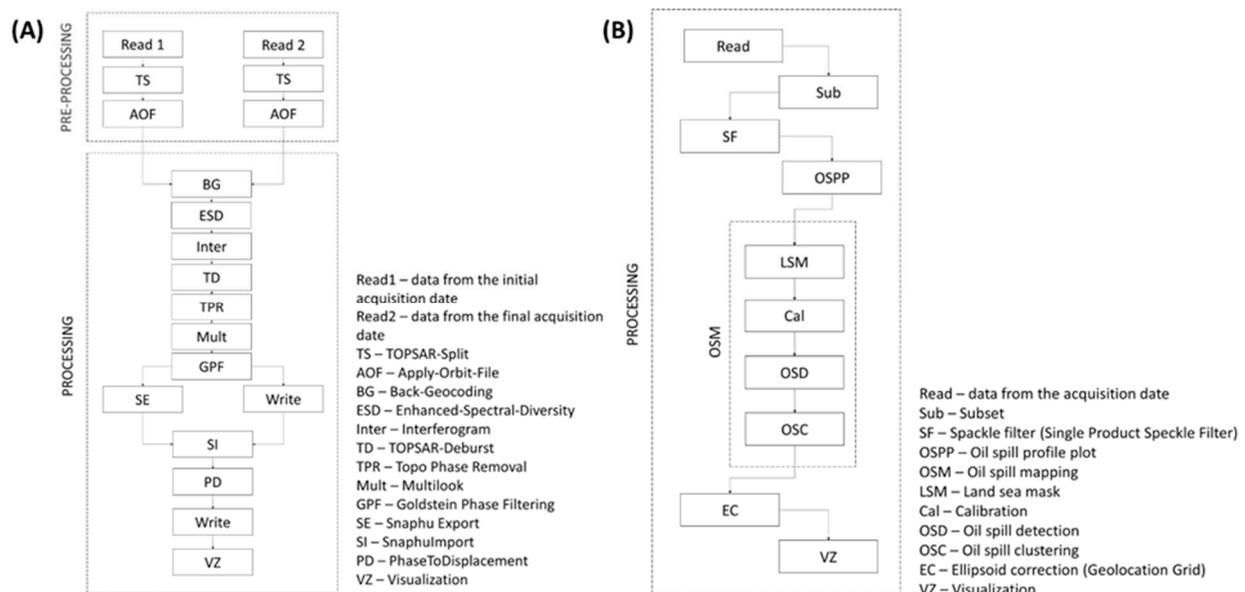
**Figure 3.** Data processing algorithms for (A) land subsidence detection and (B) oil spill detection in the SNAP tool.
