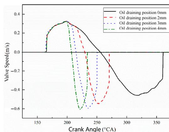
**Figure 5.** Valve velocity curves with different time of early-releasing oil.
