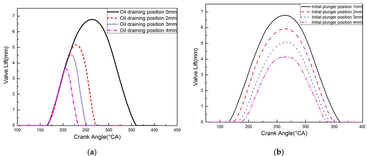
Figure 9. (a) Valve lift curve with different times of early releasing oil; (b) Valve lift curve with different times of delayed pressuring oil.
