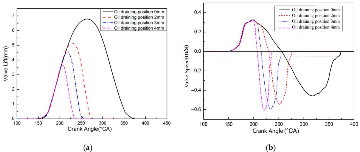
**Figure 7.** (a) Valve lift curves under different times of early-releasing oil; (b) Valve velocity curve under different times of early-releasing oil.
