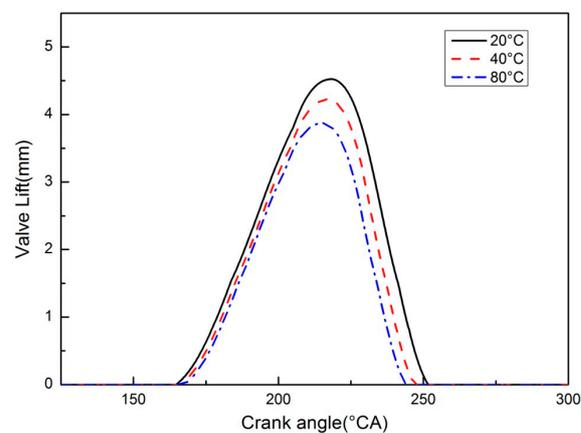
**Figure 11.** Valve lift curves at different oil temperatures.
