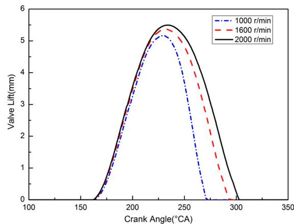
**Figure 10.** Valve lift curve at different rotational speeds.
