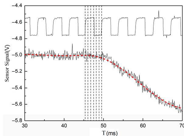
**Figure 3.** Lift and camshaft angle signals near the valve opening time.
