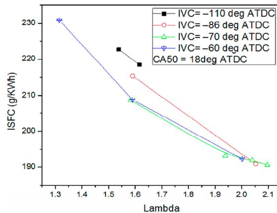
**Figure 12.** Comparison of ISFC with different intake closure angle and Lambda.
