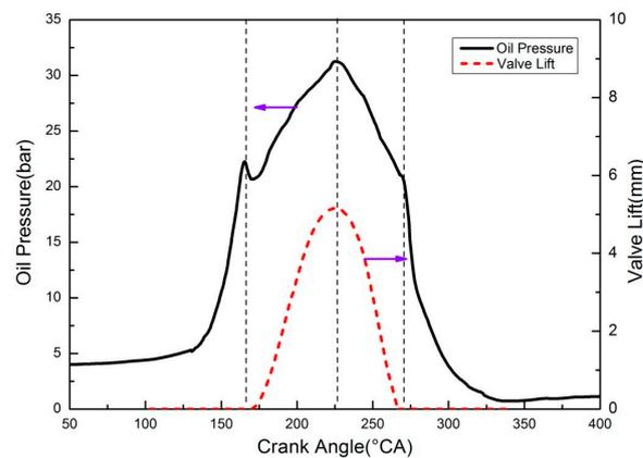
Figure 8. The relationship between valve lift and oil pressure.
