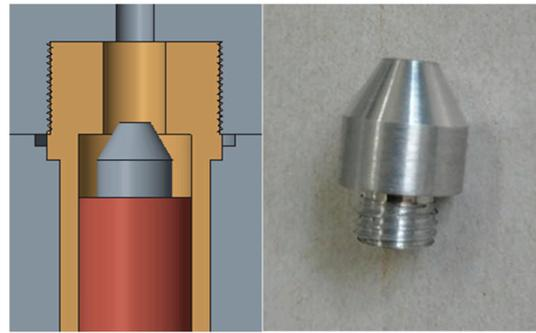
**Figure 6.** Seat buffer block.
