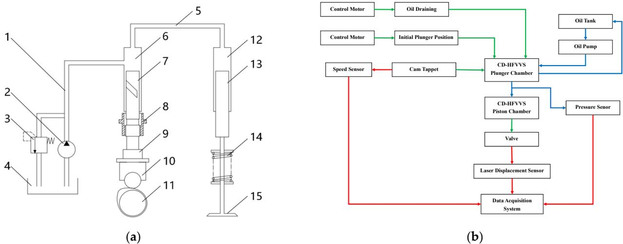
**Figure 1.** Schematic diagram of valve mechanism experiment, including (a) CD-HFVS mechanism sketch: 1. Low Pressure Oil Ducts, 2. Low Pressure Oil Pump, 3. Relief Valve, 4. Hydraulic Tank, 5. High Pressure Oil Ducts, 6. Plunger Chamber, 7. Plunger, 8. Plunger Rotary Sleeve, 9. Plunger Seat, 10. Tappet, 11. Camshaft, 12. Piston Chamber, 13. Piston, 14. Valve Spring, and 15. Valve; and (b) experimental schematic diagram.
