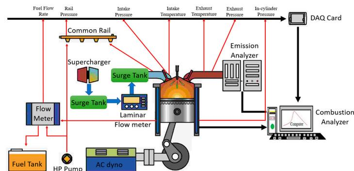
**Figure 4.** High-speed HD diesel engine and the schematic of test setup.
