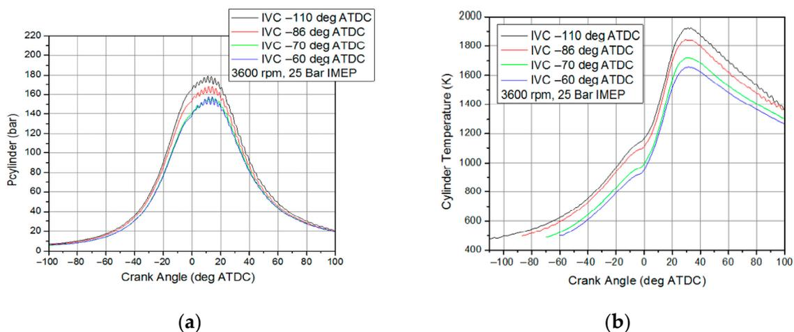
**Figure 13.** (a) Comparison of cylinder pressure with different intake closure angles; (b) Comparison of cylinder temperature with different intake closure angles.
