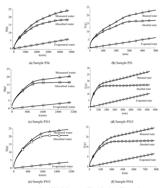
circulars, and the actual water absorption of rock sample  $Q_3$  (absorbed water), as shown in the curve with squares. Therefore, the relation of these three can be expressed as:
