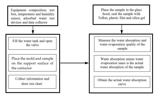
Figure 3. Real-time monitoring experimental procedures for imbibition test without water pressure.
