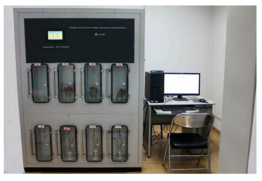
**Figure 1.** Physical experimental system for real-time experimental monitoring for water absorption evolution behaviors of sandstone in Mogao Grottoes, China.
