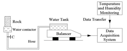
Figure 2. Sketch for real-time monitoring experimental system for imbibition test without water pressure.
