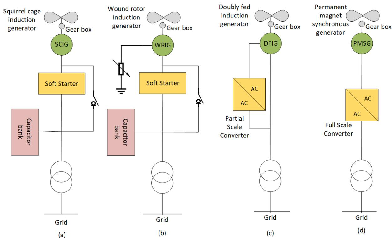
Figure 3. Grid interfacing configurations of WTGs (a) Type 1, (b) Type 2, (c) Type 3, and (d) Type 4.
