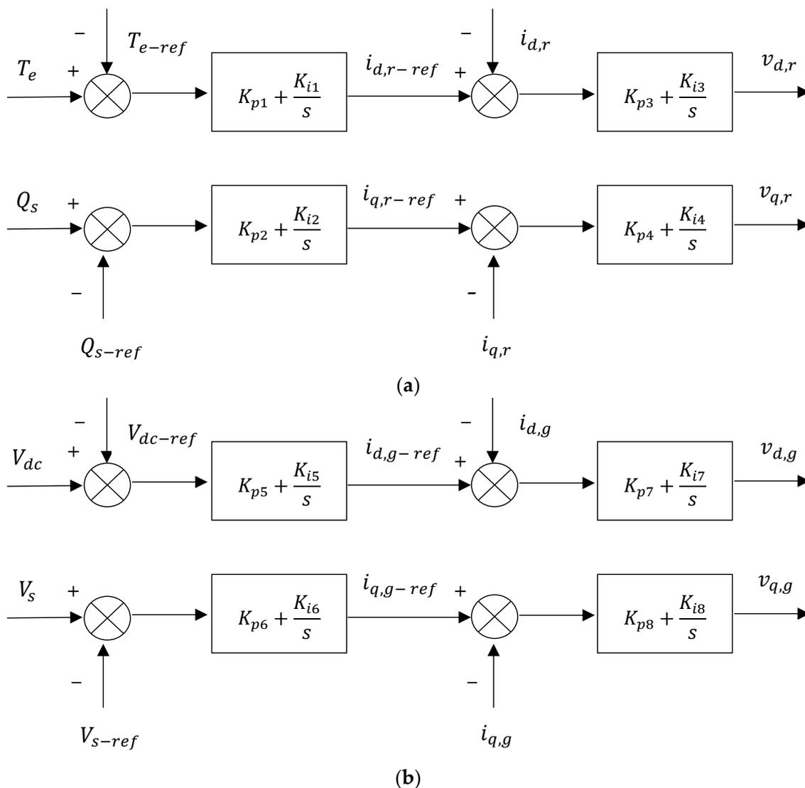
Figure 5. DFIG converter control system: (a) RSC control, (b) GSC control.
