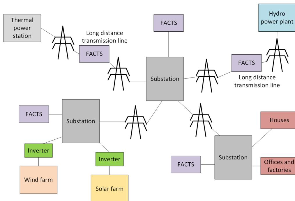
**Figure 1.** System level diagram of the modern power grid.
