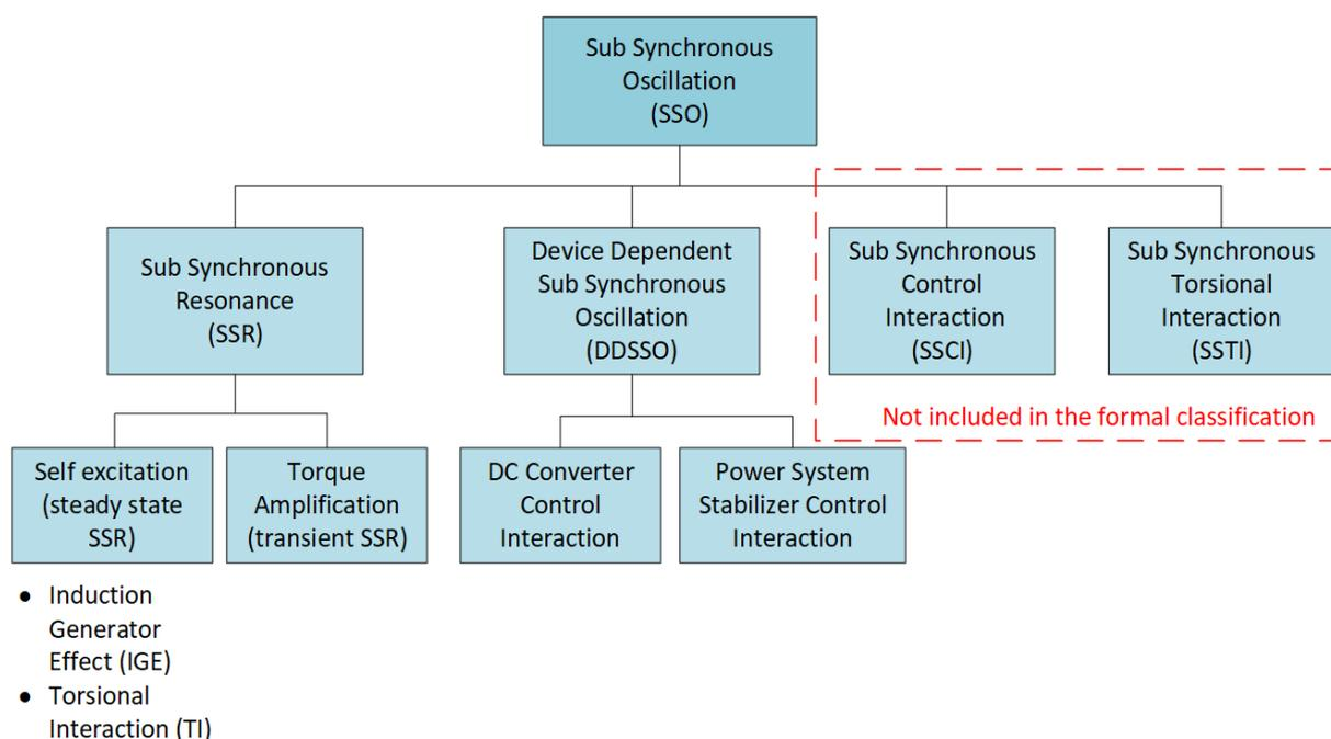
**Figure 2.** Extended classification of sub synchronous oscillation.
