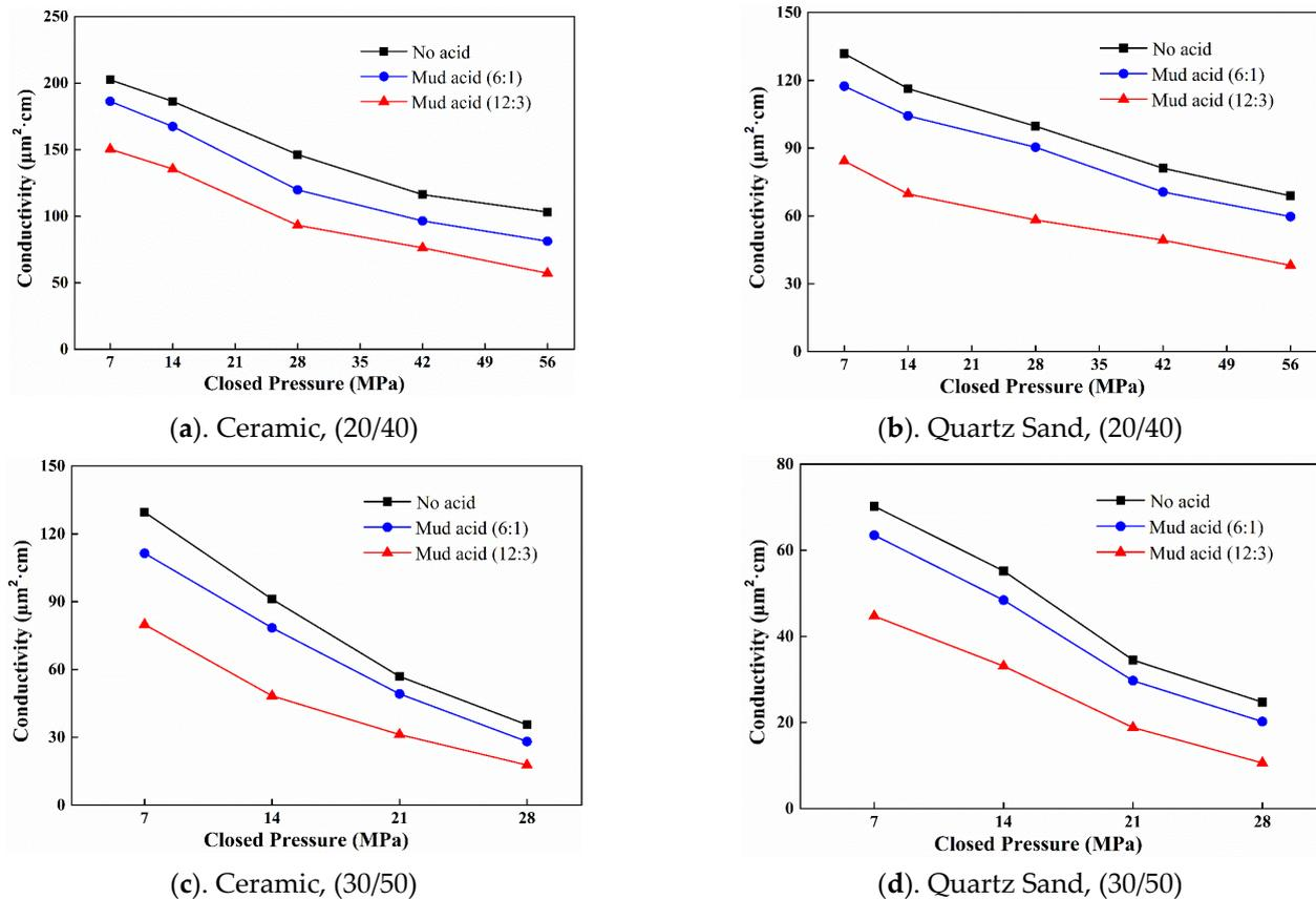
**Figure 4.** (a–d) The conductivity of ceramic and quartz sand of different sizes under different closure pressures after mud acid soaking.
