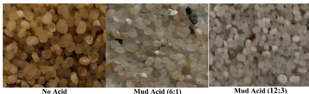
**Figure 3.** Photomicrograph of proppant after mud acid soaking experiment.
