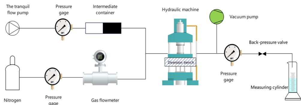
**Figure 2.** The schematic diagram of the long-term conductivity test system.
