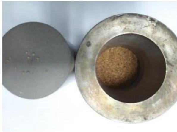
**Figure 1.** Standard crushing chamber.
