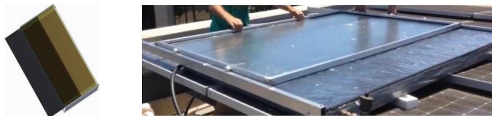
**Figure 1.** (left) adaptive cover concept; (right) black surface as absorber/emitter, plastic film wind-shield for night-time radiative cooling, and glass for solar collection.
