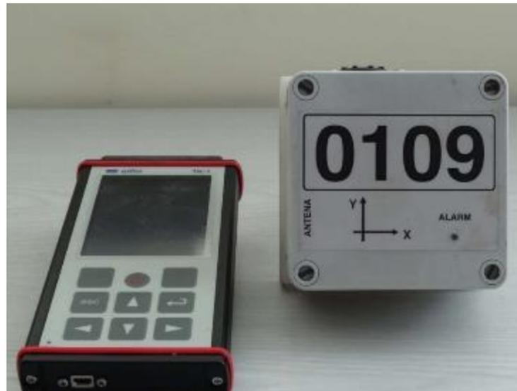
Figure 10. Inclinometric sensor with a wireless data transmitter.
