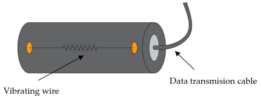
**Figure 7.** Scheme of the vibrating wire strain gauge [44].
