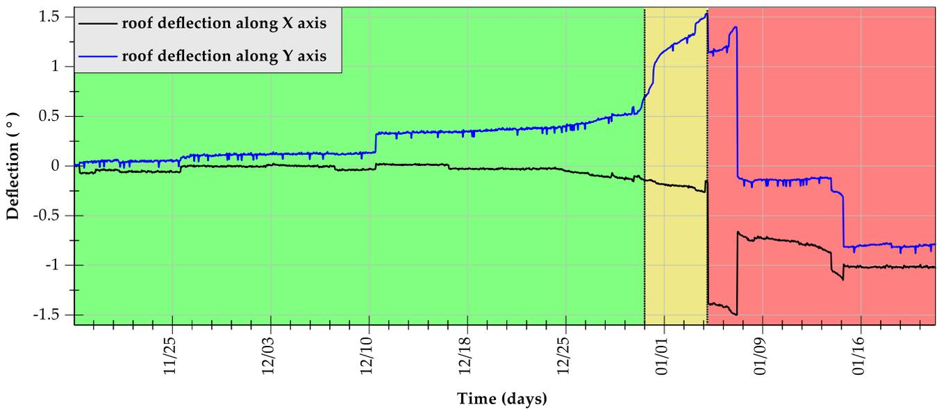
Figure 12. An exemplary case of ground failure prediction with the use of an inclinometric sensor.
