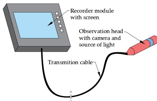
**Figure 4.** Scheme of the borehole camera system.
