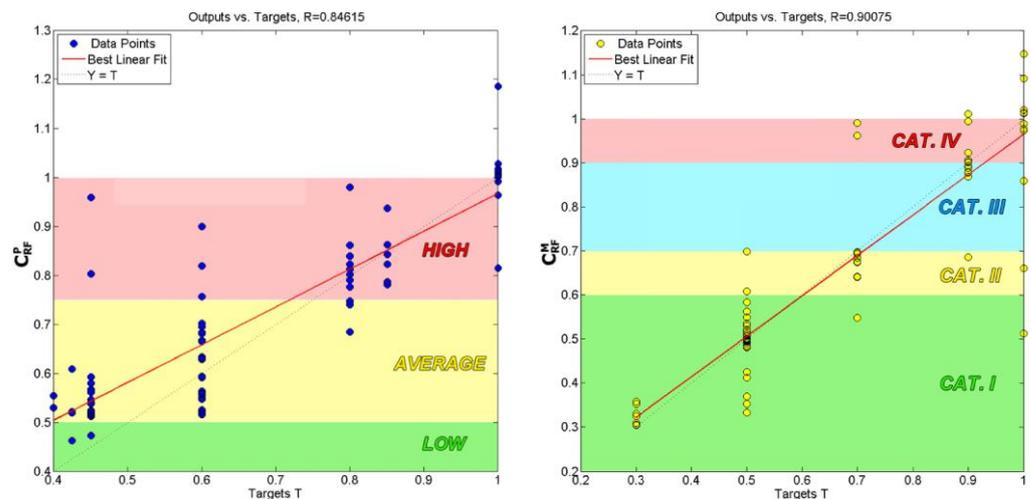
**Figure 19.** Evaluation of rock mass propensity to failure based on developed roof fall hazard index (left) and evaluation of roof stability—categories of roof fall hazard (right) [24].
