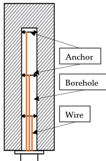
**Figure 9.** Scheme of the three point extensometer.
