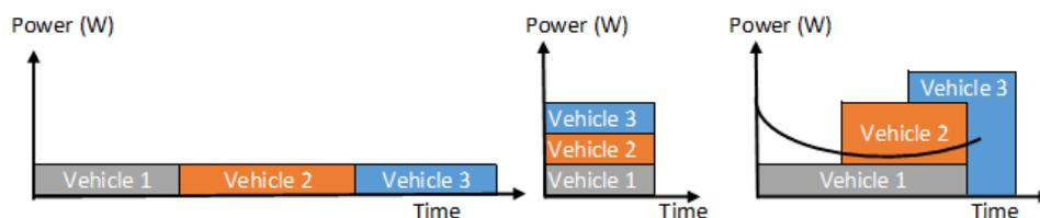
**Figure 2.** Approach to load balancing during loading.
