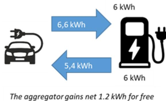
**Figure 8.** Abuse of efficiency in both directions.
