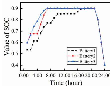
**Figure 4.** Change in SOC values of storage battery.
