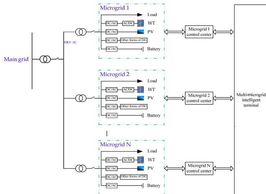
**Figure 1.** Multi-microgrid typical structure.
