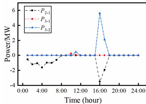
**Figure 5.** Interconnection dispatching optimization results between the two microgrids.
