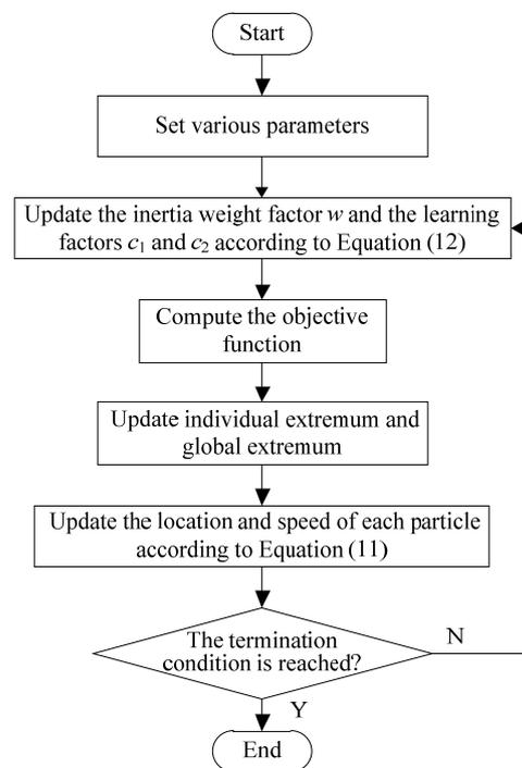
**Figure 2.** Flowchart of the solution algorithm.
