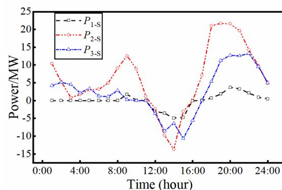
**Figure 6.** The power-dispatching optimization between the main grid and the multi-microgrid.
