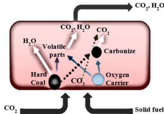
**Figure 1.** The scheme of the oxygen release process from the CLOU type of the oxygen carrier in the fuel reactor.
