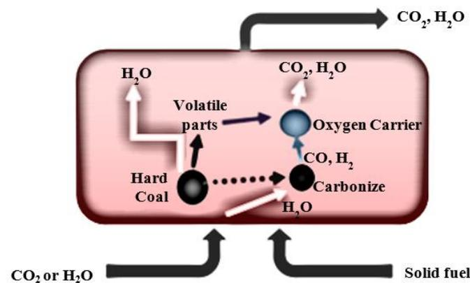
**Figure 2.** The scheme of oxygen release in the fuel reactor in the iG-CLC process.
