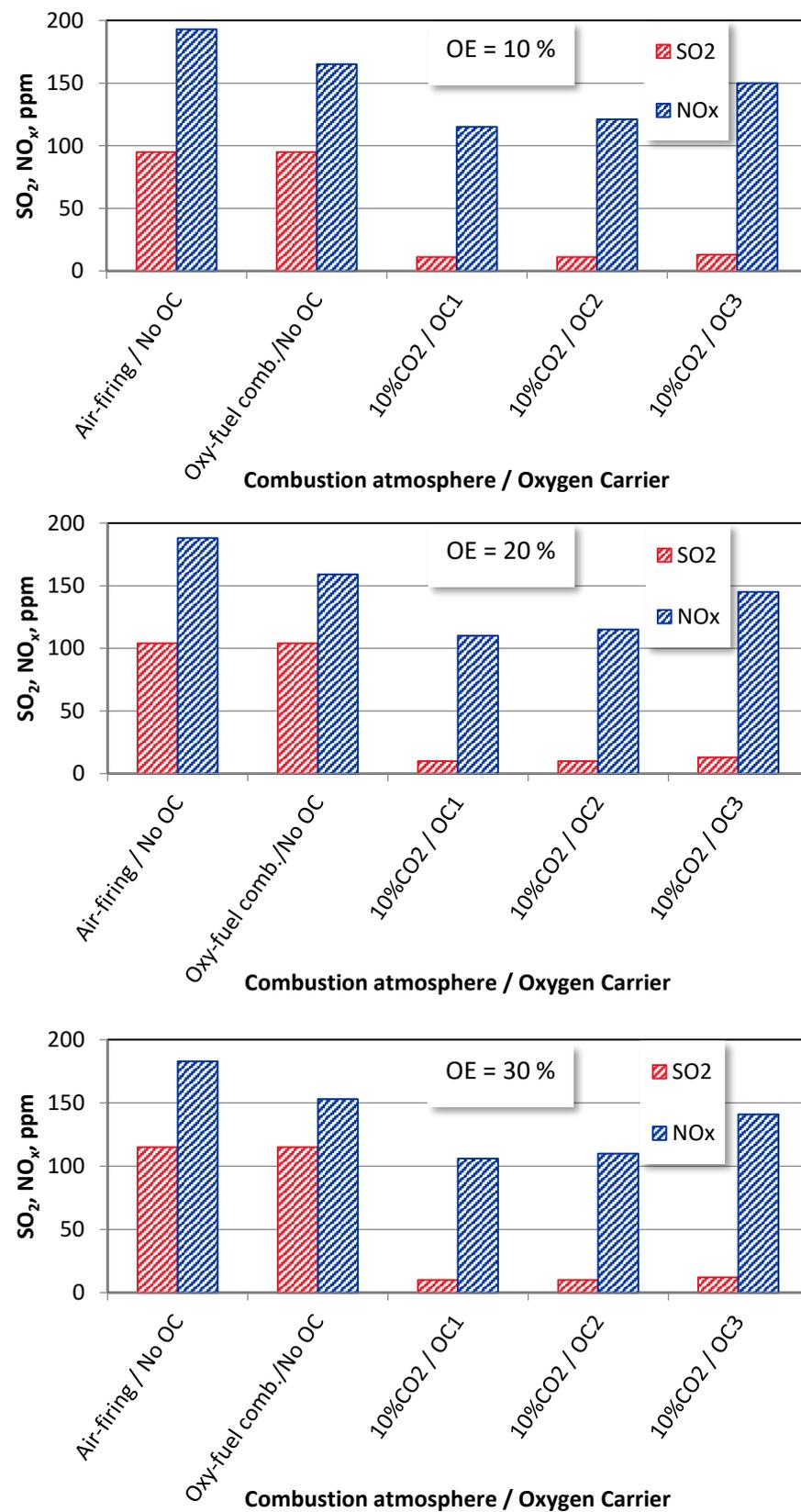
**Figure 9.** The effect of oxygen excess on SO<sub>2</sub> and NO<sub>x</sub> emissions wood chips combustion under different combustion modes (T = 1100 K).
