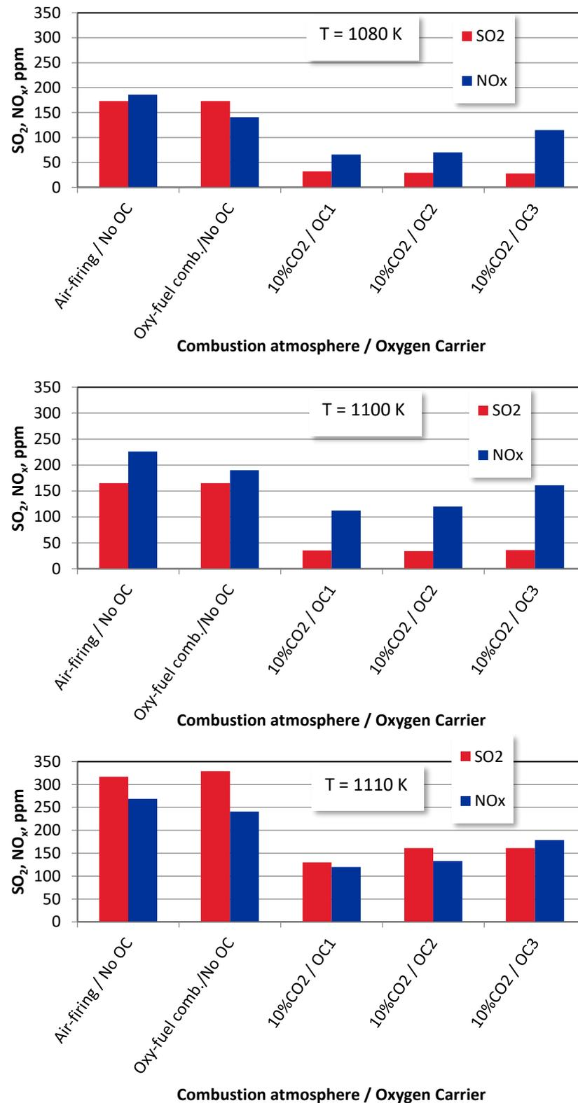
**Figure 10.** The average fuel reactor temperature effect on  $\text{SO}_2$  and  $\text{NO}_x$  emissions from bituminous coal combustion under different combustion modes (OE = 10%).
