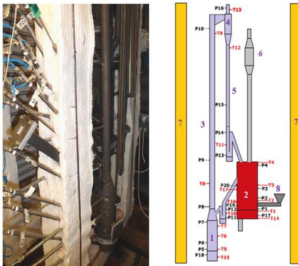
**Figure 4.** The hot FB-CLC-SF facility; 1—air reactor, 2—fuel reactor, 3—riser, 4—cyclone, 5—downcomer, 6—particle's collector, 7—heaters, 8—screw feeder, P1—P19—pressure transducers, and T1–T16—thermocouples [15].
