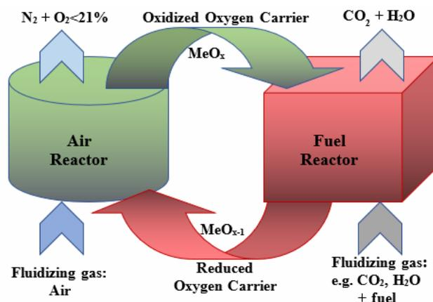
**Figure 3.** The scheme of the oxidation and reduction in the oxygen carrier in the reactors.
