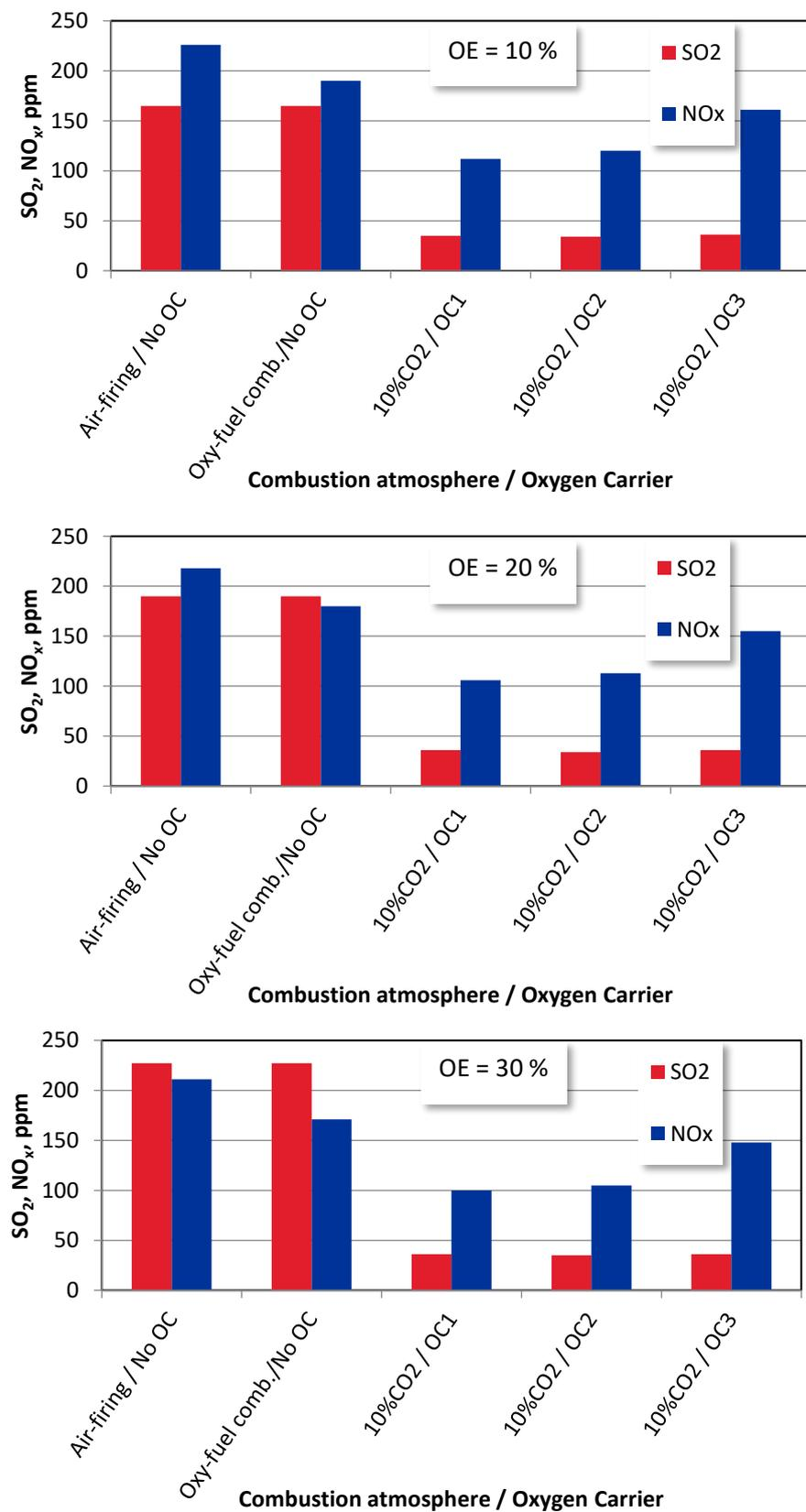
**Figure 8.** The effect of oxygen excess on SO<sub>2</sub> and NO<sub>x</sub> emissions from bituminous coal combustion under different combustion modes (T = 1100 K).
