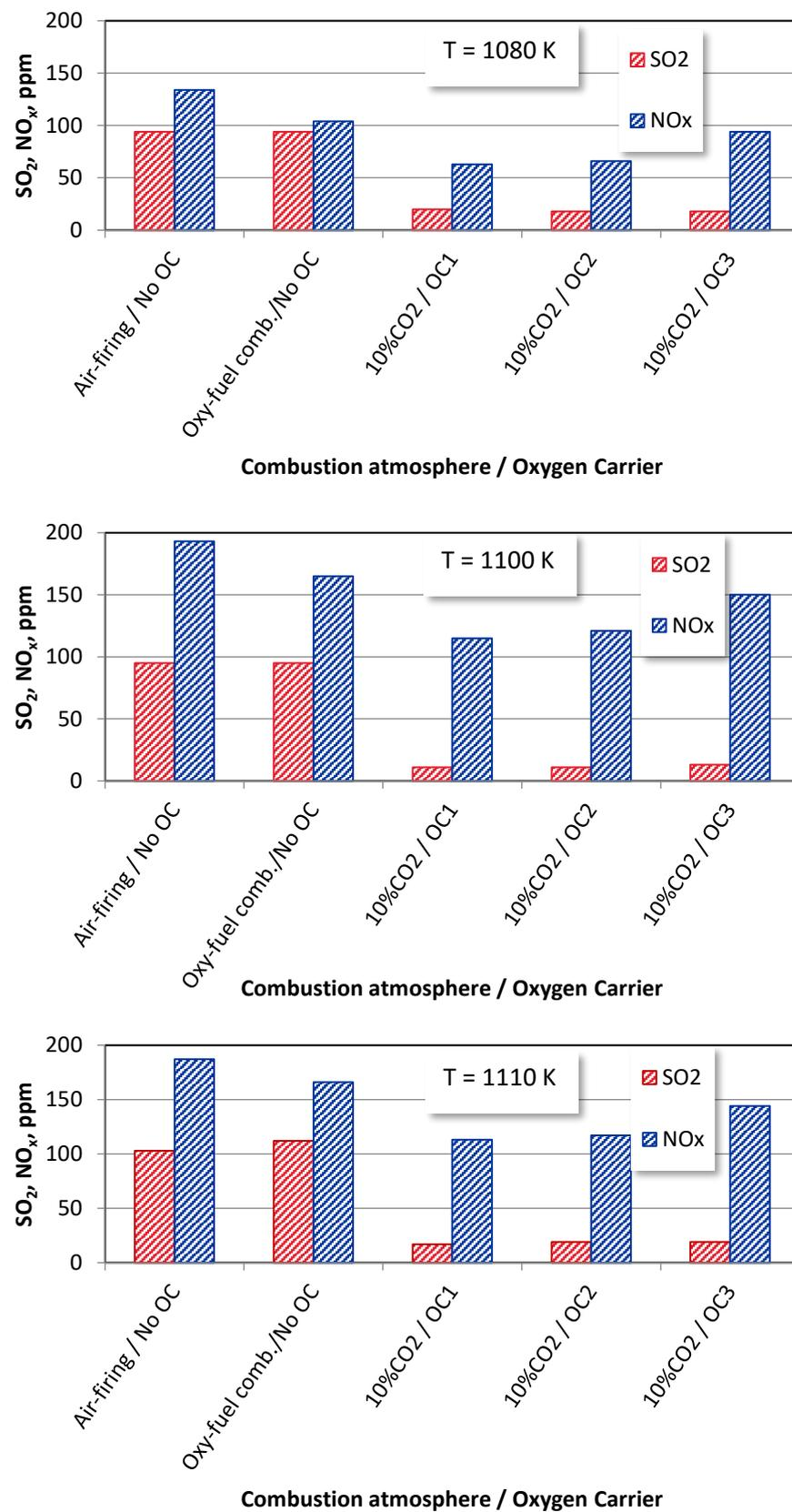
**Figure 11.** The effect of average fuel reactor temperature on SO<sub>2</sub> and NO<sub>x</sub> emissions from wood chips combustion under different combustion modes (OE = 10%).
