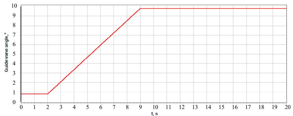
**Figure 9.** The GV opening angle versus time ( $\alpha$ ).
