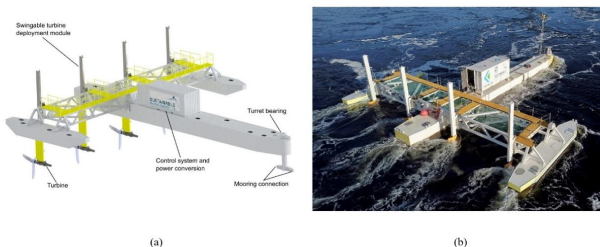
**Figure 3.** Example of a turbine array (a) CAD-model of the tidal energy converter system PLAT-I (b) Full-scale tests in Western Scotland, UK [56].
