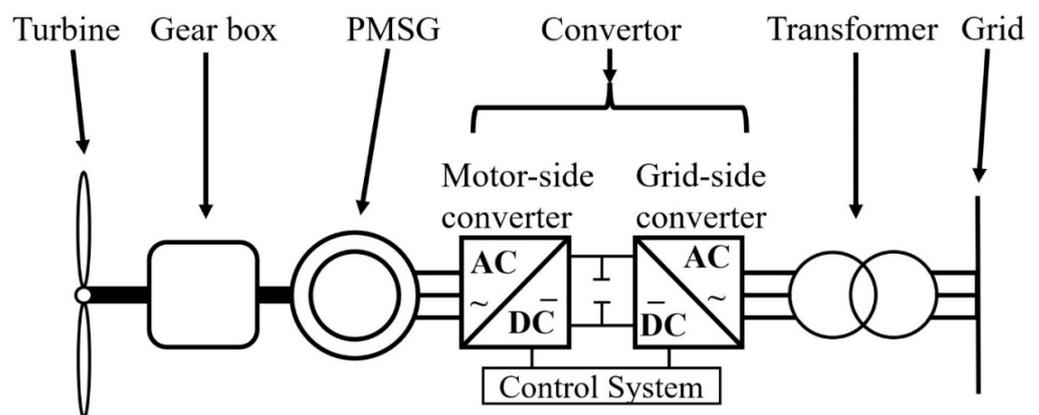
Figure 9. PMSG-based tidal TCG system.
