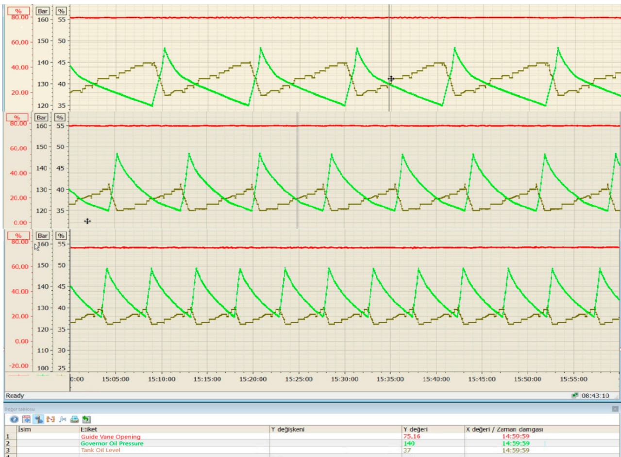
Figure 2. An example of failure in a governor hydraulic unit without any warning.
