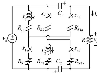
Figure 7. Proposed circuit with series losses through inductors and transistors.
