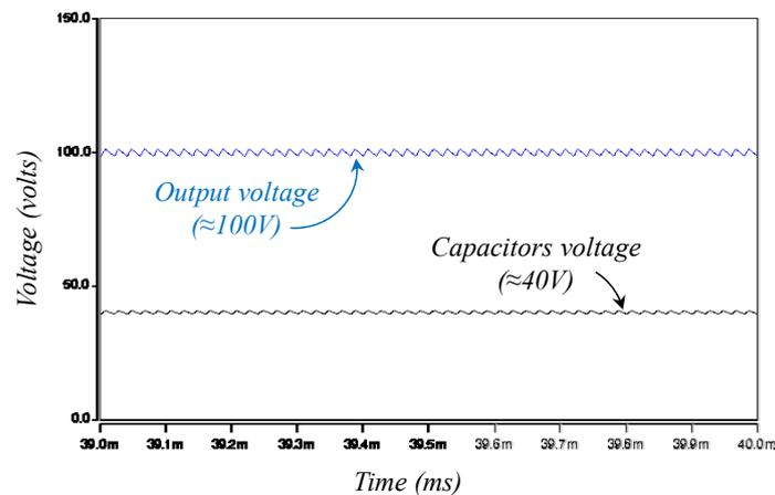
Figure 13. Output voltage and the voltage across capacitors.
