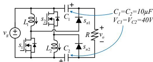
Figure 11. Solution with the proposed topology.
