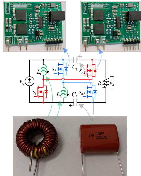
Figure 15. Experimental prototype diagram and main part photos.
