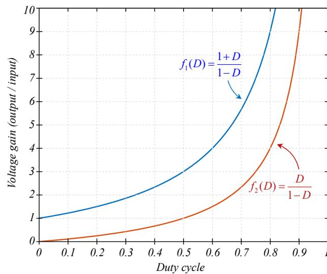
**Figure 6.** Voltage gains as a function of the duty cycle for the proposed and traditional boost converters.
