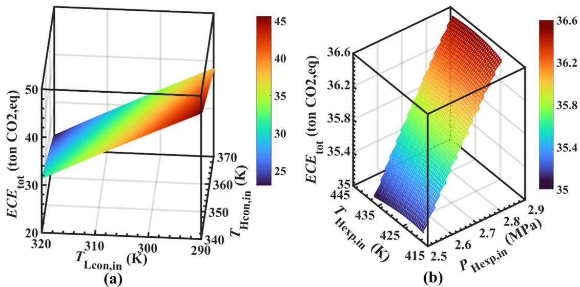
**Figure 19.** Influence characteristics of key variables on ECE. (a) Impact characteristics of condenser inlet temperature on system ECE. (b) Impact of expander inlet temperature and pressure on the HT cycle on system ECE.
