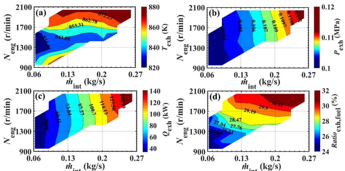
**Figure 4.** Waste heat characteristics of exhaust in variable working environments. (a) Inlet temperature of exhaust. (b) Temperature different of exhaust. (c) Heat transfer rate of exhaust. (d) Proportion of heat transfer rate in exhaust.
