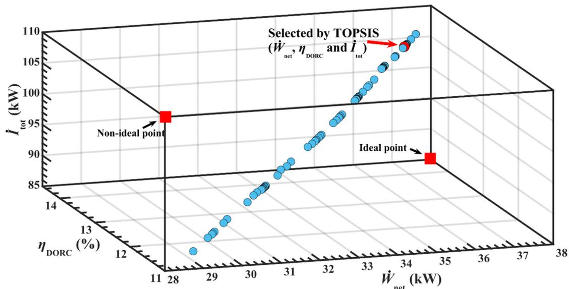
Figure 20. Multi objective optimization and TOPSIS selection.
