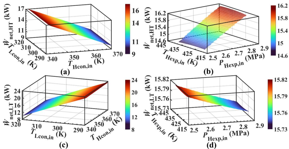
**Figure 6.** Influence characteristics of key variables on power in HT cycle and LT cycle. (a) Influence characteristics of different loop condenser inlet temperatures on HT cycle power. (b) Impact characteristics inlet temperature and the pressure of the expander on the power in the HT cycle. (c) Effect characteristics of different loop condenser inlet temperatures on LT cycle power. (d) Effect of expander parameters of the HT cycle on the power of the LT cycle.
