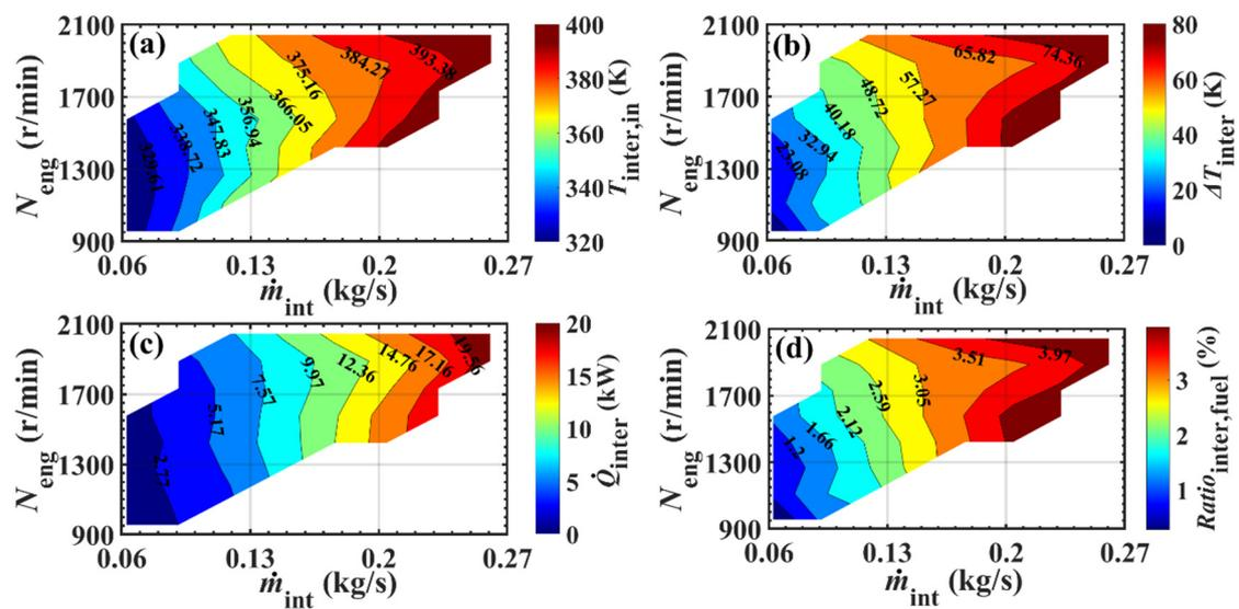
**Figure 2.** Waste heat characteristics of intercooler in variable working environments. (a) Inlet temperature of intercooler. (b) Temperature different of intercooler. (c) Heat transfer rate of intercooler. (d) Proportion of heat transfer rate in intercooler.
