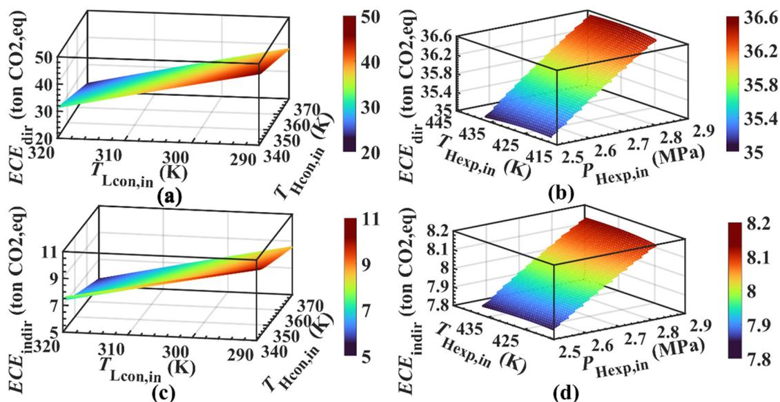
**Figure 18.** Influence characteristics of key variables on direct ECE and indirect ECE. (a) Effect characteristics of the inlet temperature of the condenser in different loops on direct ECE. (b) Effect characteristics of the expander on the HT cycle direct ECE. (c) Effect characteristics of the inlet temperature of the condenser in different loops on indirect ECE. (d) Effect characteristics of the expander on the HT cycle indirect ECE.
