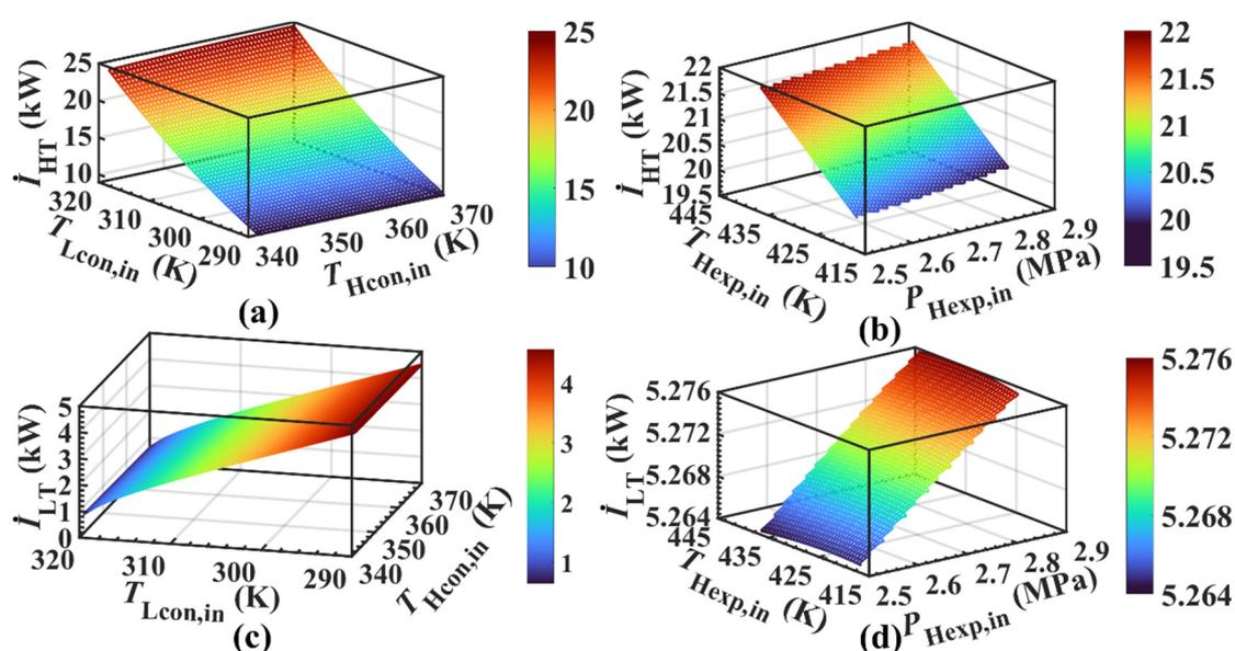
**Figure 15.** Influence characteristics of key variables on exergy destruction of HT cycle and LT cycle. (a) Effect of exergy destruction in the HT cycle. (b) Effect of exergy destruction in the HT cycle. (c) Effect of exergy destruction in the LT cycle. (d) Effect characteristics of exergy destruction in the HT cycle.
