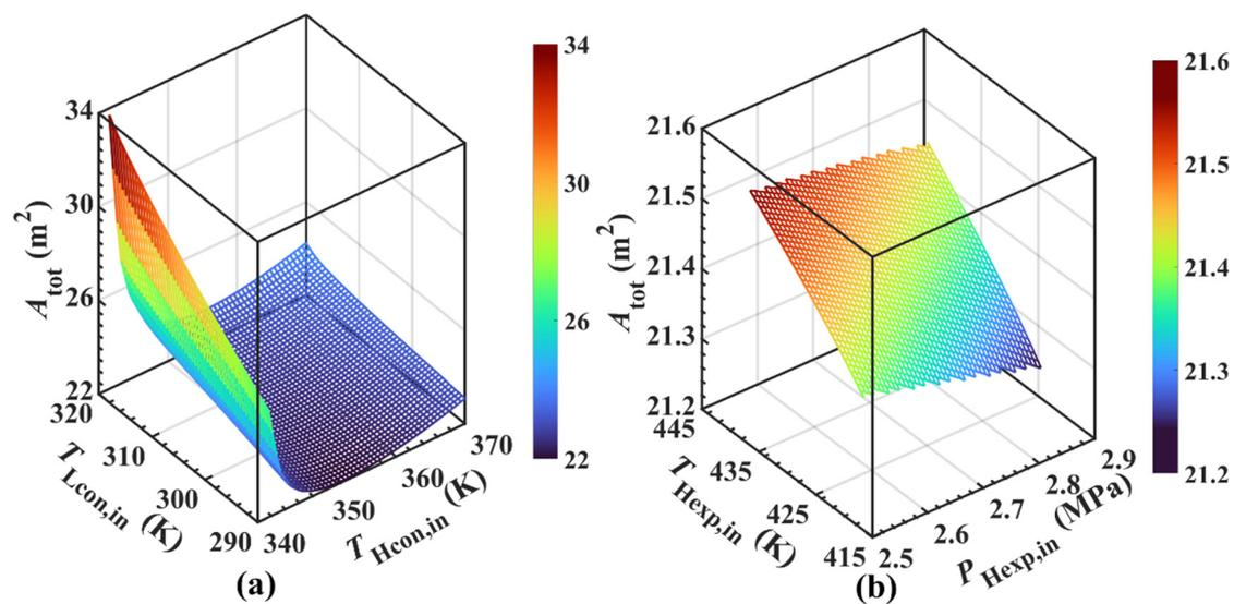
**Figure 10.** Influence characteristics of key variables on the system heat transfer surface. (a) Effect characteristics of inlet temperature in a condenser on the system heat transfer surface in the HT cycle and the LT cycle. (b) Effect characteristics of the parameters of the expander in the HT cycle on the system heat transfer surface.
