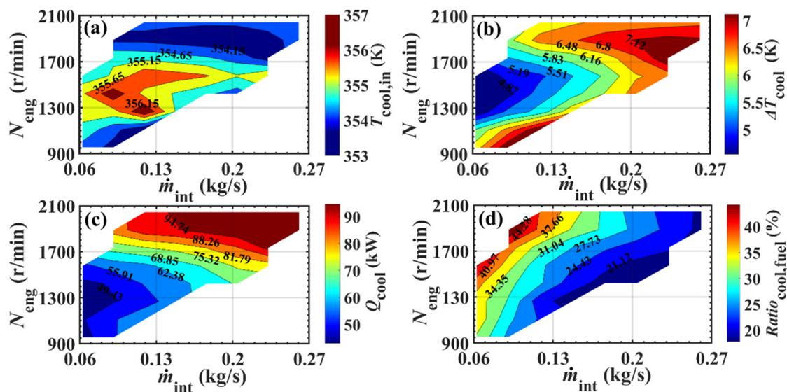
**Figure 3.** Waste heat characteristics of coolant in variable working environments. (a) Inlet temperature of coolant. (b) Temperature different of coolant. (c) Heat transfer rate of coolant. (d) Proportion of heat transfer rate in coolant.
