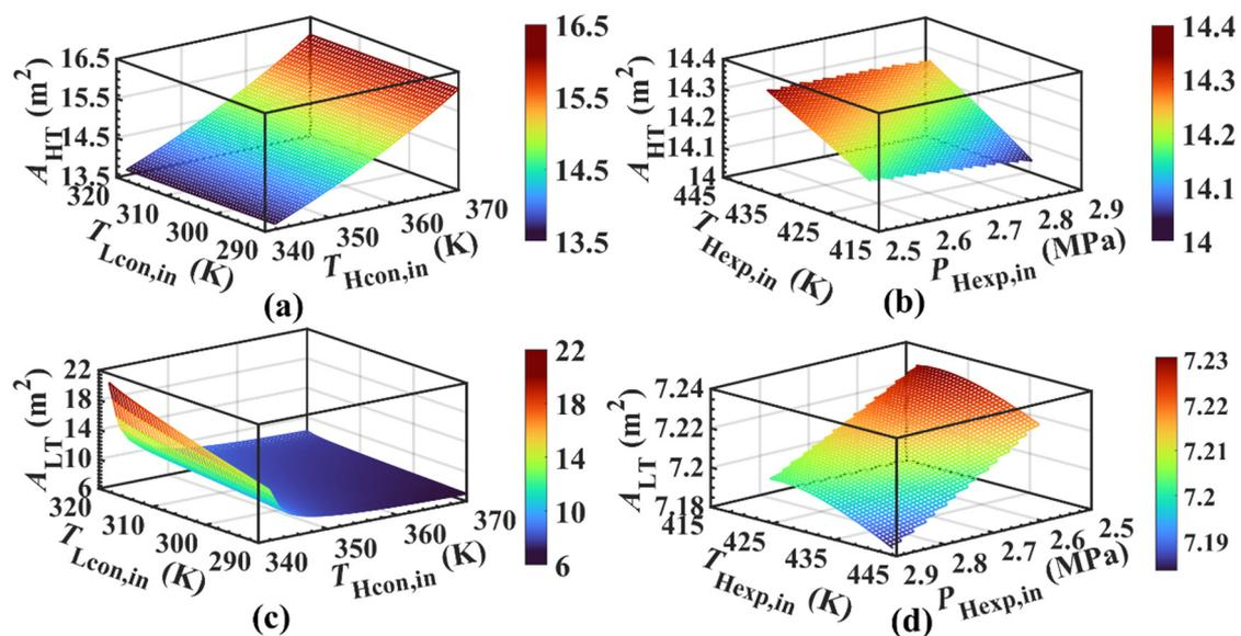
**Figure 9.** Influence characteristics of key variables on the heat transfer surface of the HT cycle and the LT cycle. (a) Effect the characteristics in the condenser inlet temperature of different loops on the heat transfer surface for the HT cycle. (b) Effect characteristics of heat transfer surface in the HT cycle. (c) Effect characteristics in different loops on the heat transfer surface of the LT cycle. (d) Effect characteristics of the heat transfer surface of the LT cycle.
