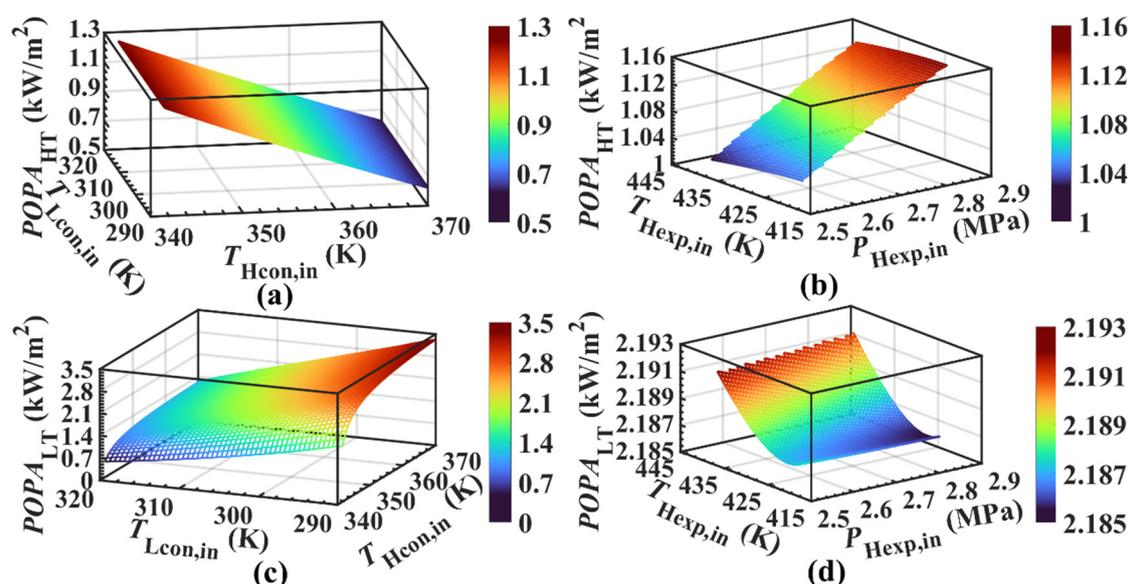
**Figure 12.** Influence characteristics of key variables on POPA of HT cycle and LT cycle. (a) POPA effect characteristics of the condenser inlet temperature in different loops on the HT cycle. (b) Effect characteristics of POPA in the HT cycle. (c) POPA effect characteristics on the LT cycle. (d) Effect characteristics on the HT cycle.
