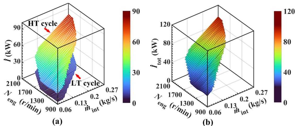
**Figure 14.** Exergy destruction of HT cycle, LT cycle and the system under variable working conditions. (a) Exergy destruction characteristics of different cycles. (b) System exergy destruction characteristics.
