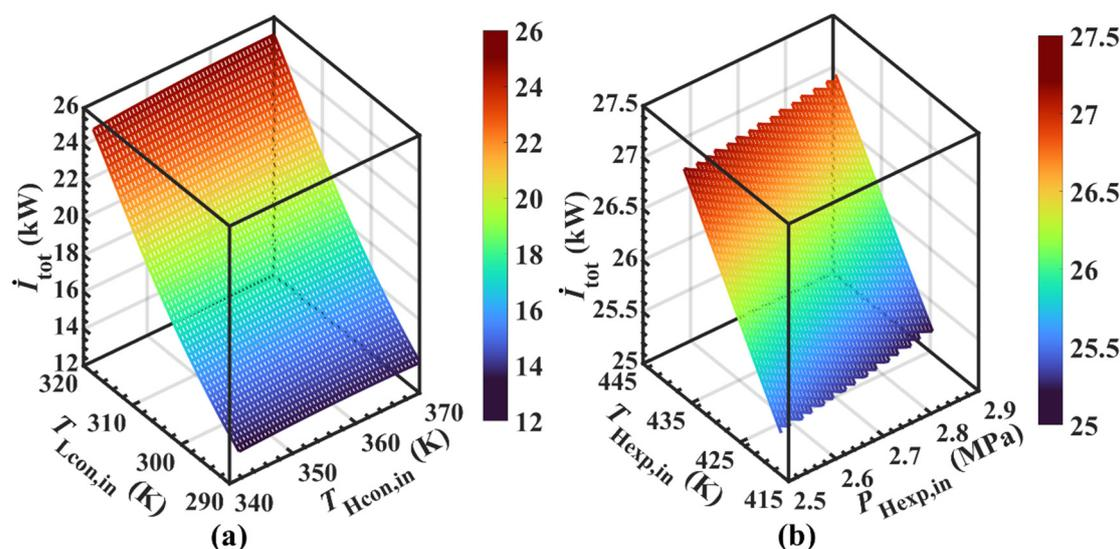
**Figure 16.** Influence characteristics of key variables on exergy destruction. (a) Effect characteristics of condenser inlet temperature in different cycles on exergy destruction. (b) Effect characteristics of inlet temperature and pressure of the expander of the HT cycle for system exergy destruction.
