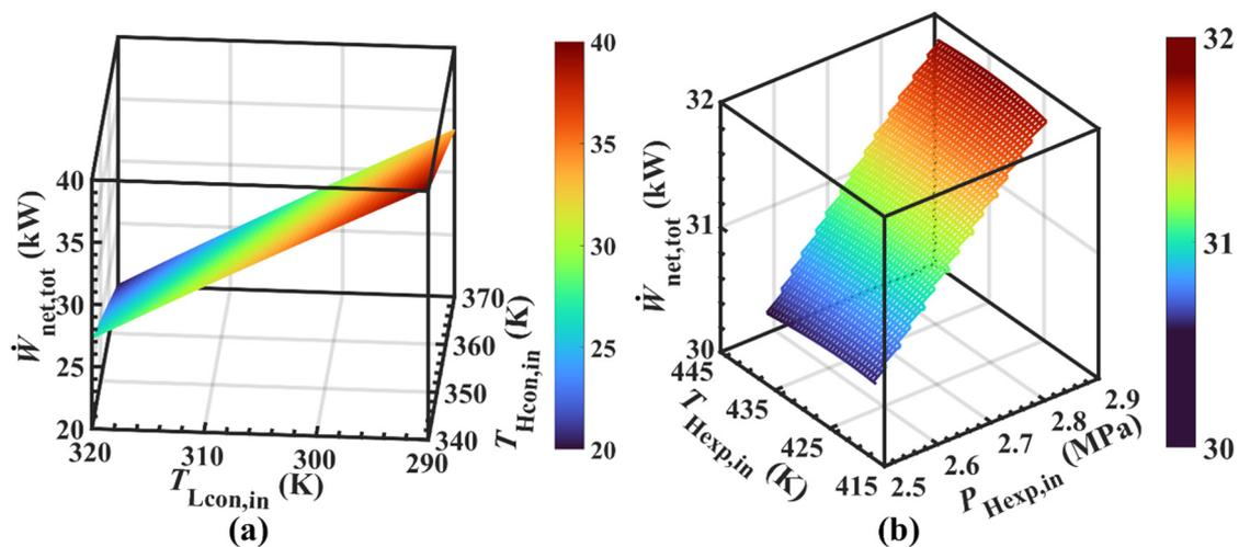
**Figure 7.** Influence characteristics of key variables on system power output. (a) Effect characteristics of inlet temperature of a condenser on the system power in a different cycle. (b) Effect characteristics of parameter of expander on system power in HT cycle.
