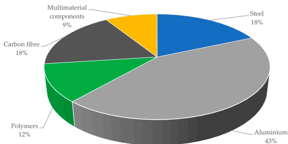
**Figure 3.** Percentage breakdown by weight of the materials that make up the analysed e-cargo bike.
