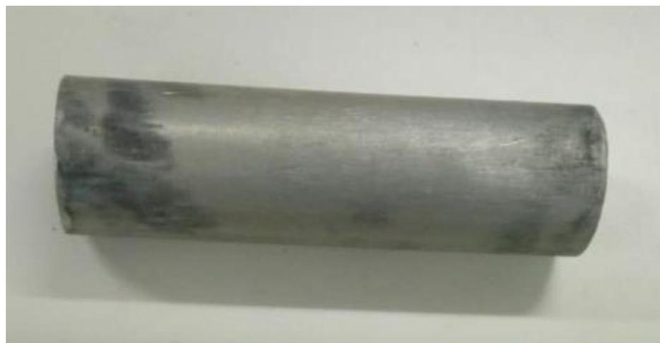
**Figure 22.** Armature for the dynamic test.
