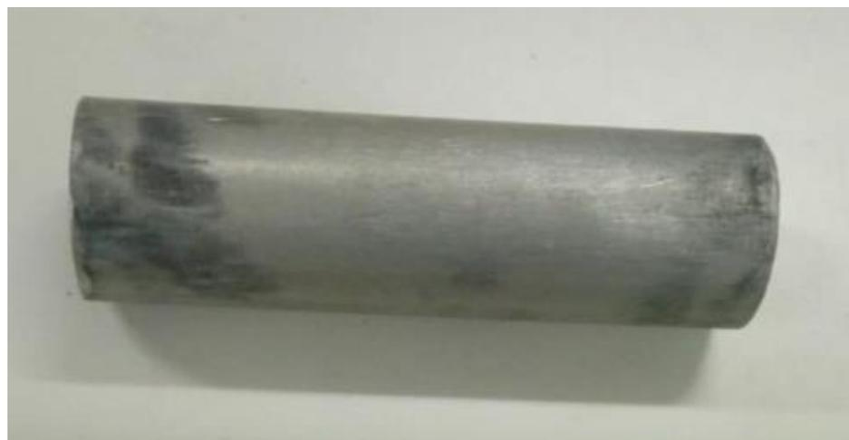
**Figure 22.** Armature for the dynamic test.
