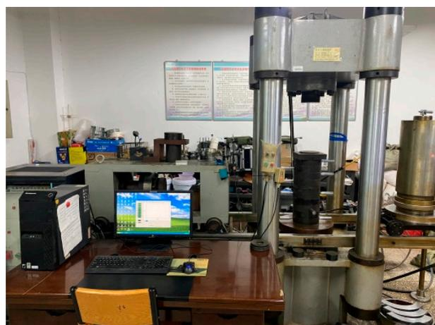
**Figure 3.** RLW-2000 rock triaxial rheology servo rheometer.
