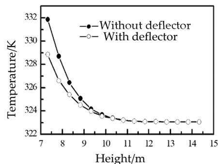
**Figure 13.** Average temperature of a representative section with and without deflector.
