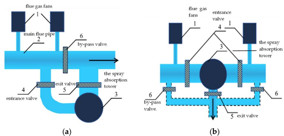
**Figure 2.** The layout of flue gas desulfurization tower; (a) Single inlet; (b) Dual inlet. 1—flue gas fans; 2—main flue pipe; 3—the spray absorption tower; 4—entrance valve; 5—exit valve; 6—by-pass valve.
