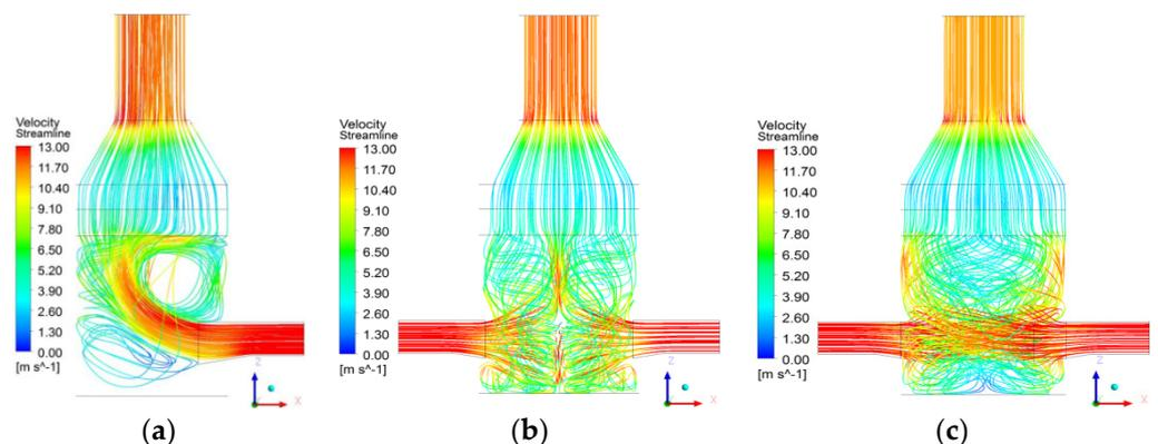
**Figure 4.** The gas phase streamlines without spray; (a) Single inlet; (b) Straight dual inlet; (c) Tangential dual inlet.
