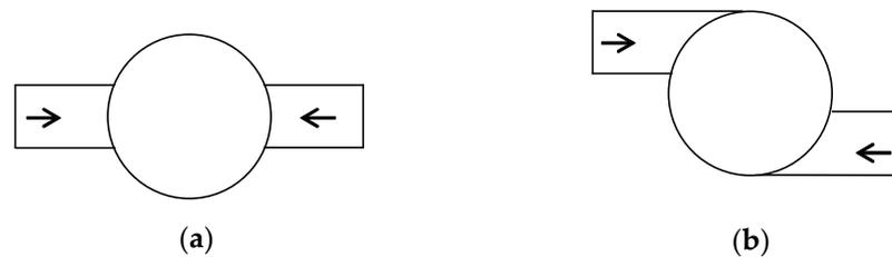
**Figure 3.** Vertical view of tower with Dual inlet; (a) Straight dual inlet; (b) Tangential dual inlet.
