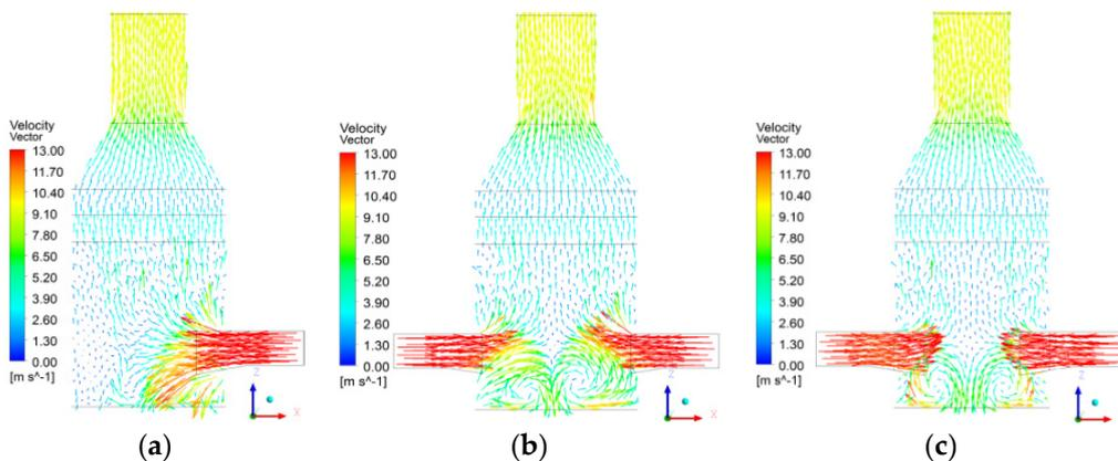
**Figure 6.** The gas velocity vector diagram with spray; (a) Single inlet; (b) Straight dual inlet; (c) Tangential dual inlet.
