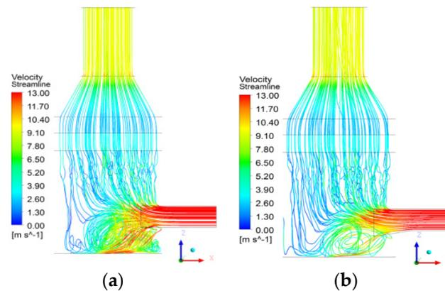
**Figure 7.** The gas phase streamlines diagram with and without flue baffle; (a)  $d = 0$  m; (b)  $d = 0.5$  m.
