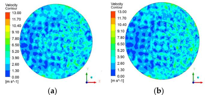
**Figure 12.** The gas velocity contours of cross-section at  $z = 1$  m under the second spray layer. (a) Without deflector; (b) With deflector.
