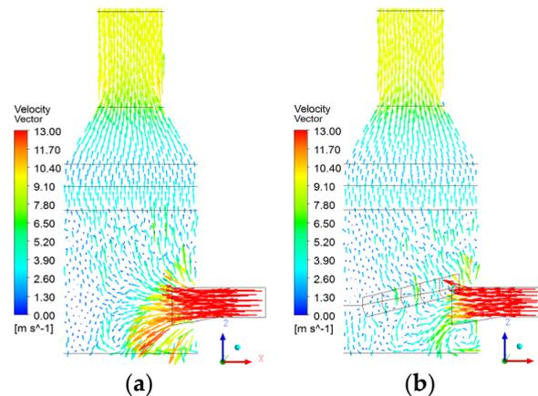
**Figure 11.** The gas velocity vector diagram with and without deflector; (a) Without deflector; (b) With deflector.
