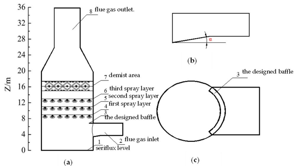
**Figure 1.** Diagrammatic sketch of the desulfurization spray tower; (a) tower structure; (b) flue gas inlet angle; (c) designed baffle in flue gas inlet. 1—seriflux level; 2—flue gas inlet; 3—the designed baffle; 4—first spray layer; 5—second spray layer; 6—third spray layer; 7—demist area; 8—flue gas outlet.
