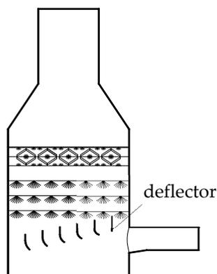
**Figure 10.** The schematic diagram of the installation of deflectors installed in the tower.
