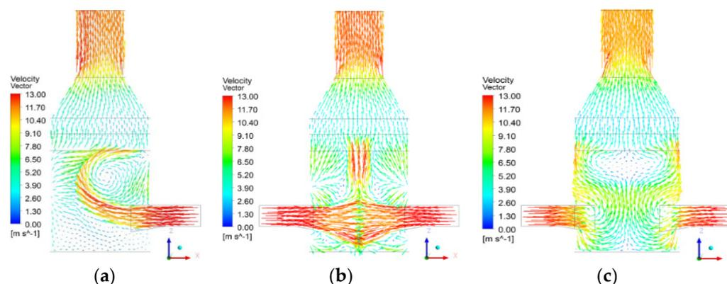
**Figure 5.** The gas velocity vector diagram without spray; (a) Single inlet; (b) Straight dual inlet; (c) Tangential dual inlet.
