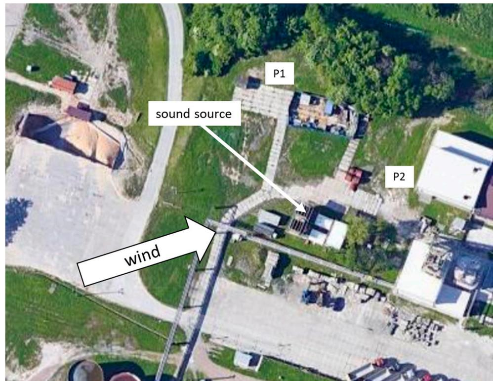
**Figure 3.** Placement of measurement points relative to the noise source. P1, P2—measurement points—source: google.maps.com.
