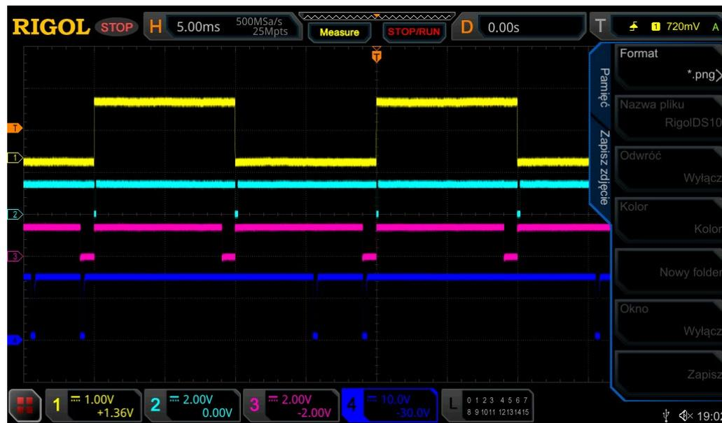
Figure 16. Synchronization signals of the RMF rectifier in the energy recovery circuit.
