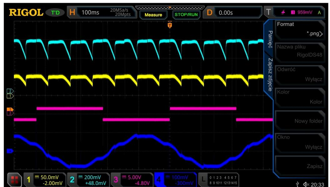
Figure 15. Current, voltage, synchronization signal and phase-to-phase voltage waveforms in the RMF rectifier.
