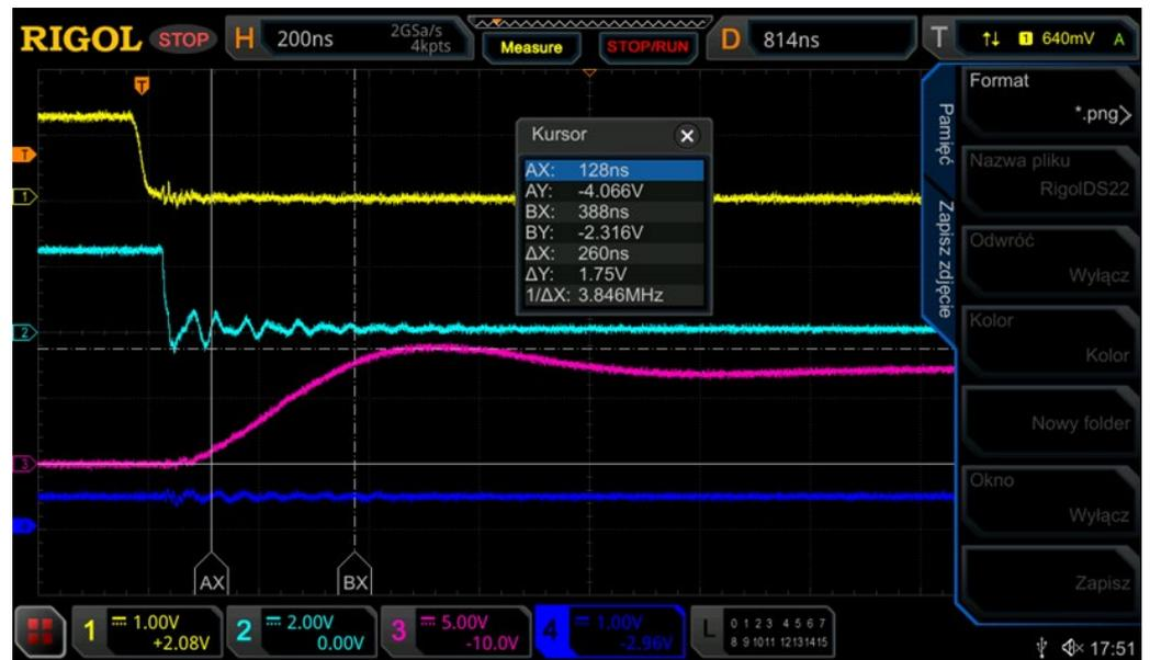
Figure 14. Oscillogram of the 260 ns gate pulse rising slope  $di_g/dt$ .
