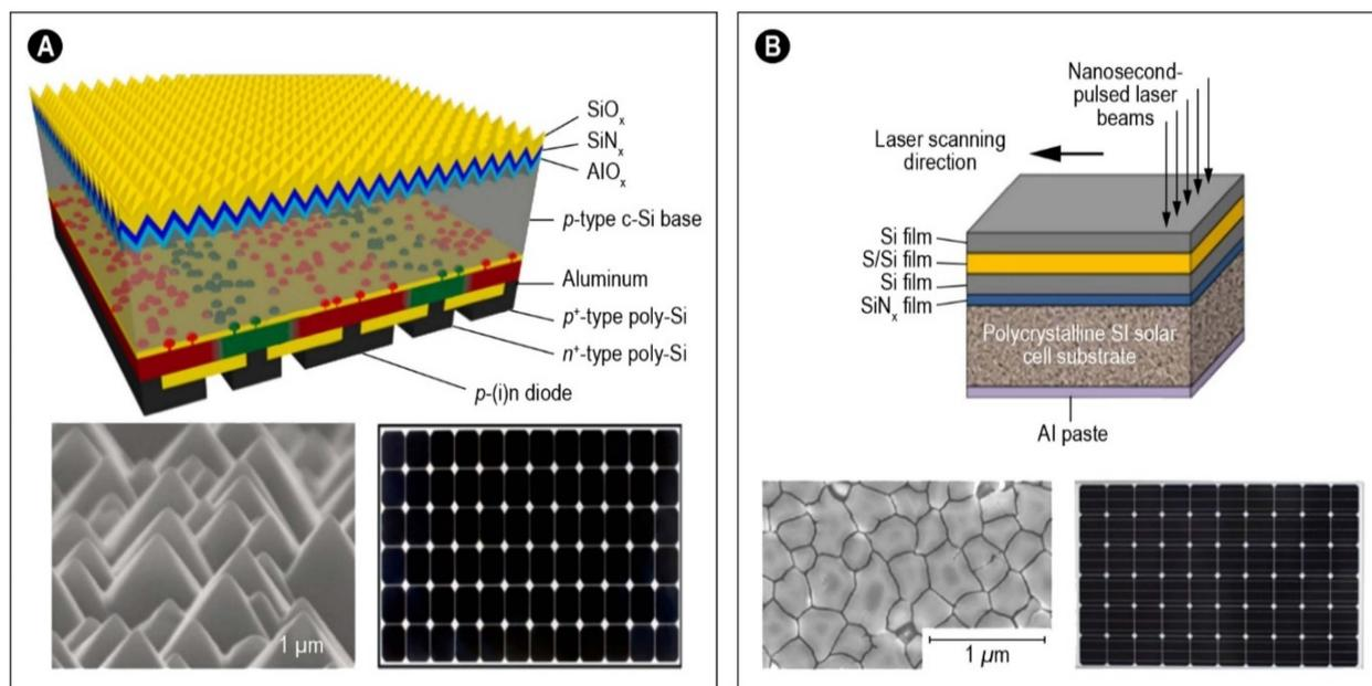
**Figure 5.** (A) Representative images of monocrystalline solar cell structure, scanning electron micrograph, and physical appearance of a monocrystalline solar module [74–76]; (B) a typical polycrystalline solar cell, scanning electron micrograph, and physical appearance of a polycrystalline solar module [77,78].
