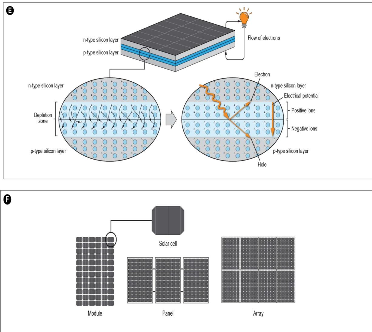
**Figure 2.** (A) Parabolic-trough solar concentrator [12,13]; (B) Parabolic dish collector [23,24]; (C) Solar power tower system [25]; (D) Schematic diagram of solar cell [32,33]; (E) A solar cell n-type and p-type layers [35–37]; and (F) Schematic of solar cell, module, panel, and array systems [39–41].
