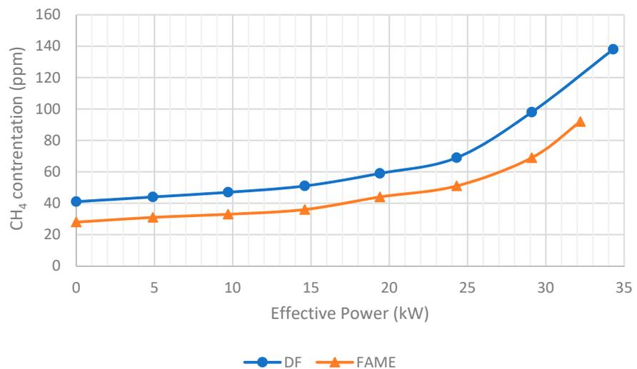
**Figure 11.** CH<sub>4</sub> emission level in the exhaust as a function of the effective power of the S-4003 engine, at an engine speed of 2200 rpm.
