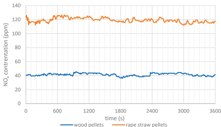
**Figure 5.** Time course of changes in  $\text{NO}_x$  concentration for combustion tests of wood pellets and rape straw pellets.
