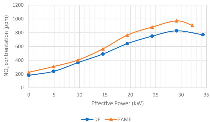
**Figure 9.** NO<sub>x</sub> emission level in the exhaust as a function of the effective power of the S-4003 engine, at an engine speed of 2200 rpm.
