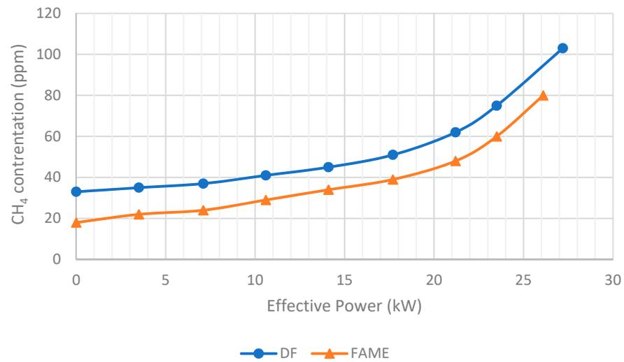
**Figure 10.** CH<sub>4</sub> emission level in the exhaust as a function of the effective power of the S-4003 engine, at an engine speed of 1600 rpm.
