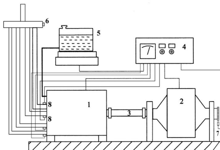
**Figure 2.** Scheme of the dynamometer stand: 1—test engine, 2—load brake, 3—shaft connecting the engine to the brake, 4—control and measurement system, 5—fuel consumption measuring system, 6—exhaust gas intake, 7—induction speed sensor, 8—exhaust gas temperature sensors.
