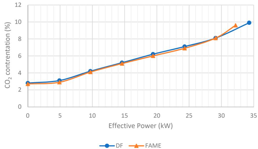
**Figure 7.** CO<sub>2</sub> emission level in the exhaust gas as a function of the effective power of the S-4003 engine, at an engine speed of 2200 rpm.
