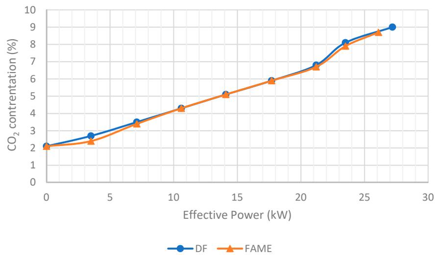
**Figure 6.** CO<sub>2</sub> emission level in the exhaust gas as a function of the effective power of the S-4003 engine, at an engine speed of 1600 rpm.
