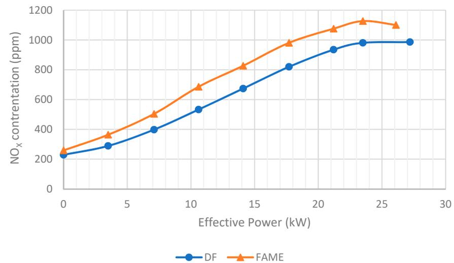
**Figure 8.** NO<sub>x</sub> emission level in the exhaust gas as a function of the effective power of the S-4003 engine, at an engine speed of 1600 rpm.
