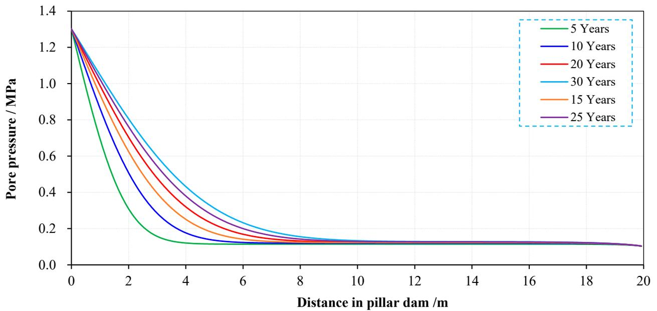
Figure 3. Distribution of pore pressure in the coal pillar of the underground reservoir with a depth of 100 m.
