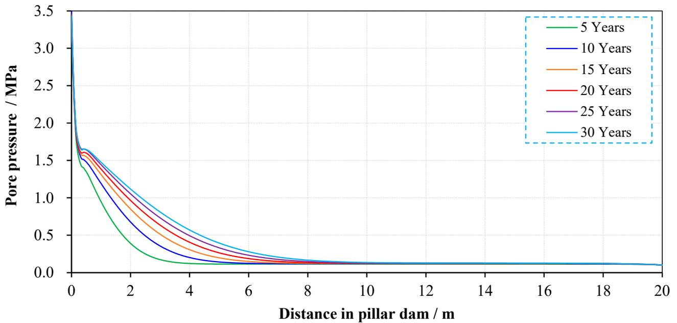
Figure 8. Distribution of pore pressure in the pillar during 30 years of operation.
