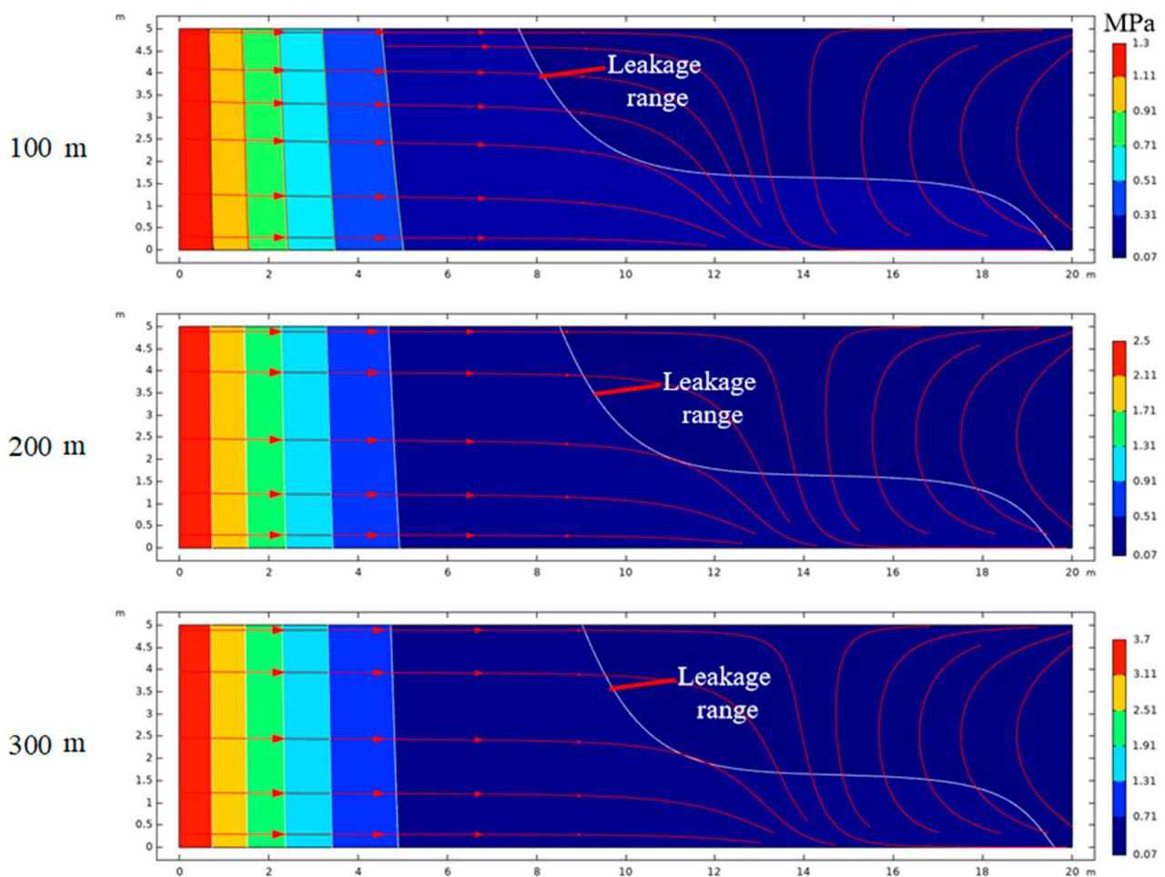
Figure 5. Distribution of seepage range in the coal pillar dam with different depths (Unit: MPa).
