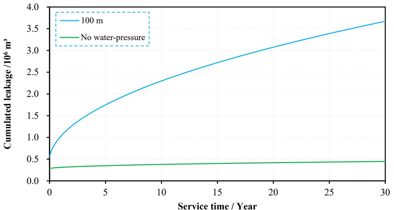
**Figure 4.** Cumulative leakage in the coal pillar of the underground reservoir.
