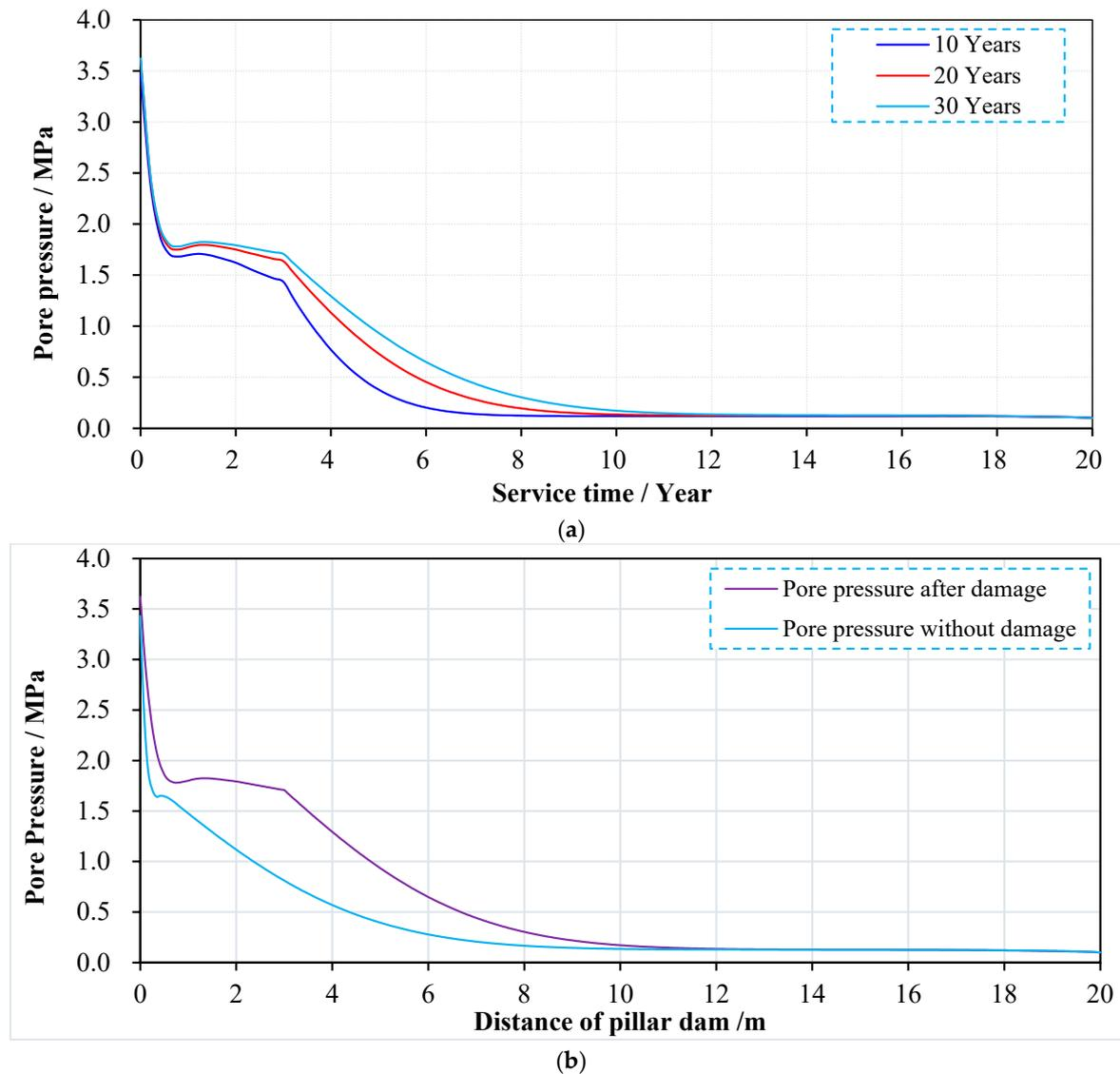
**Figure 15.** Distribution of pore pressure in the coal pillar dam. (a) pore pressure distribution of the coal pillar dam with damaged zones at different times; (b) comparison of pore pressure distribution of the damaged and undamaged coal pillar dam.
