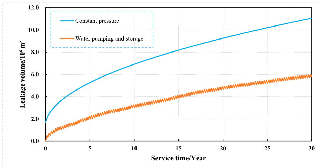
Figure 9. Cumulative leakage of reservoir with water pumping and storage.
