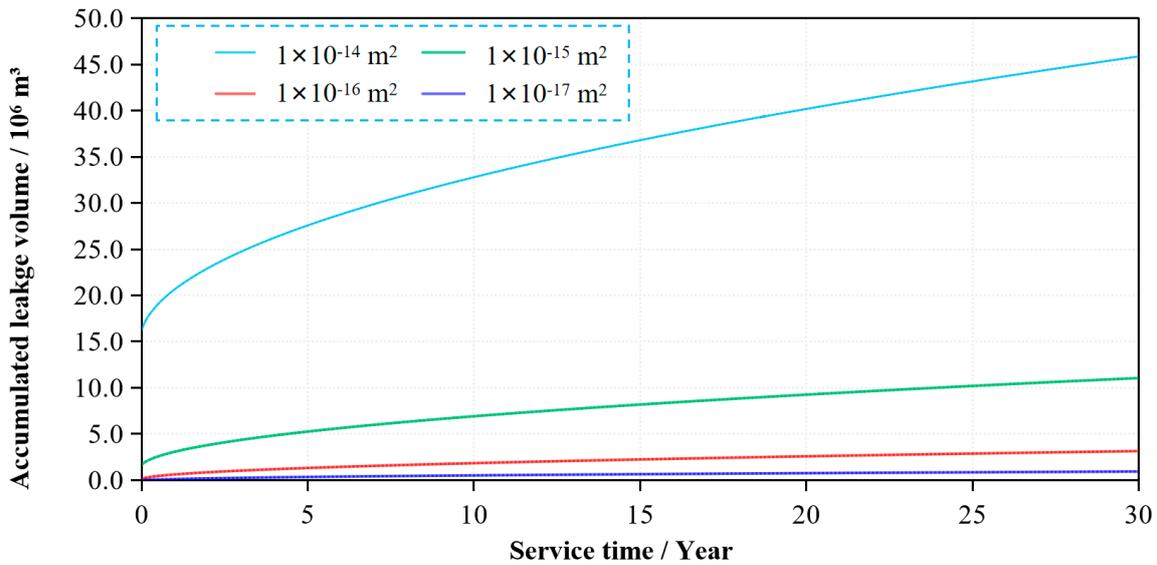
Figure 12. Cumulative water leakage amount of the coal pillar dam with different permeability.
