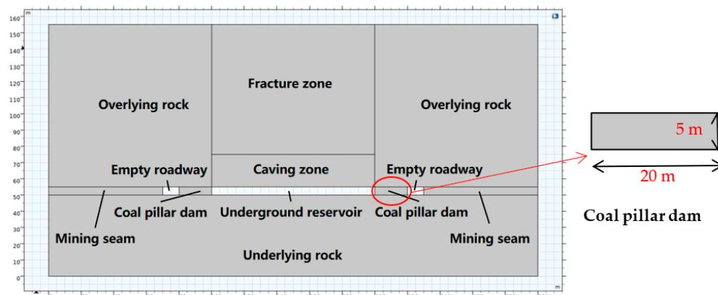
Figure 1. 2D geological model of the underground reservoir and coal pillar dam in the coal mine.
