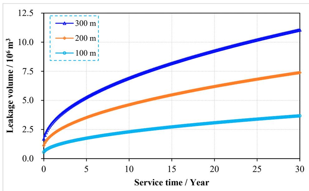
Figure 7. Accumulated leakage volume in coal pillars under different depths.
