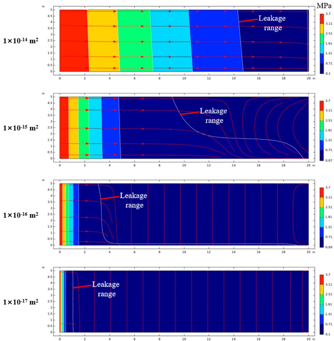
Figure 10. Leakage range and streamlining the distribution of coal pillar dam with different permeability.
