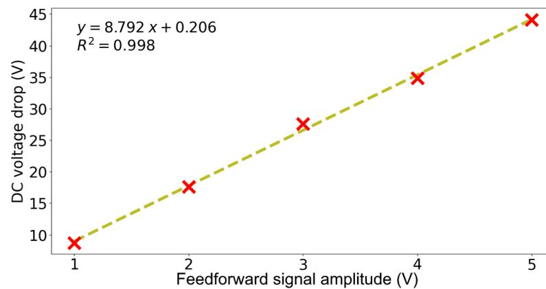
**Figure 10.** Relation between system voltage drop and feedforward signal amplitude for Cloud 2.
