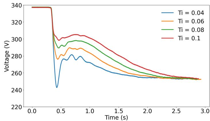
**Figure 19.** System voltage signal at the starting phase with  $K_p = 2$  and different  $T_i$ .
