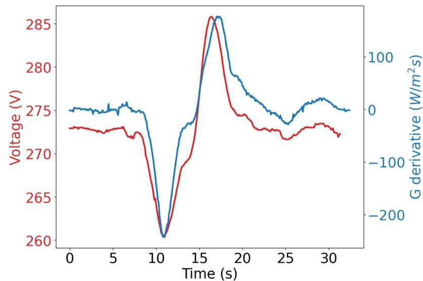
**Figure 8.** Voltage and derivative of irradiance comparison.
