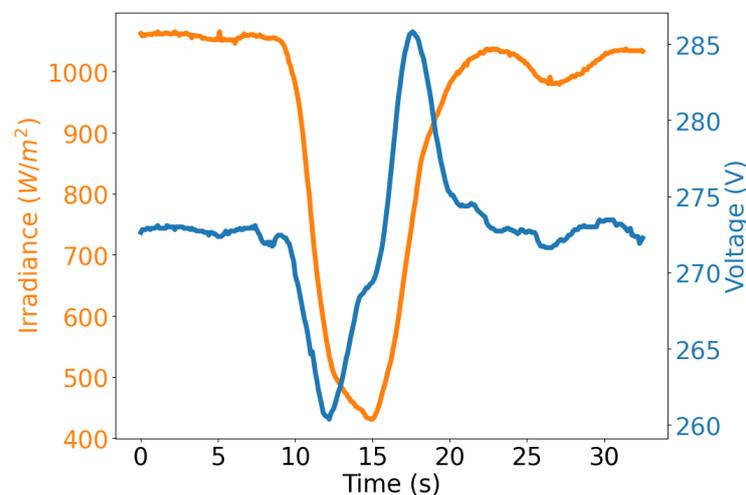
**Figure 3.** Cloud 2 (59.41% irradiance drop): irradiance fluctuation and corresponding system voltage disturbance.
