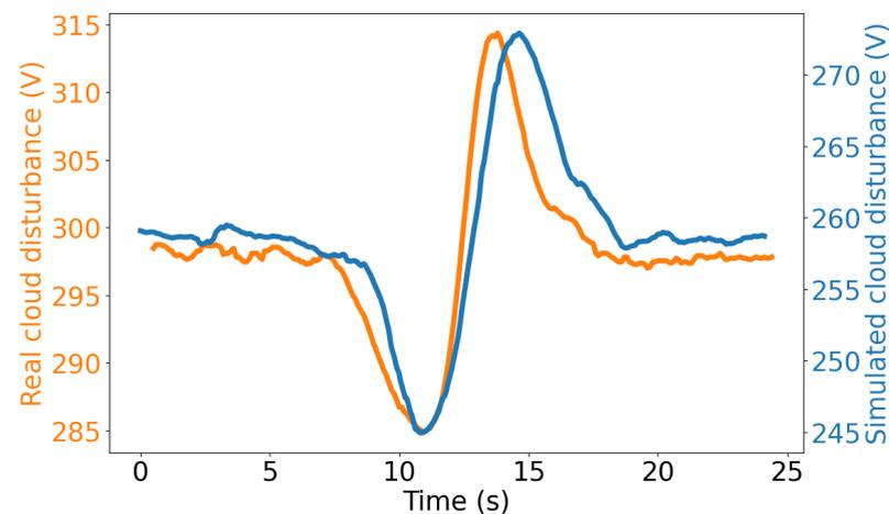
**Figure 13.** System voltage disturbance with real and simulated Cloud 1.
