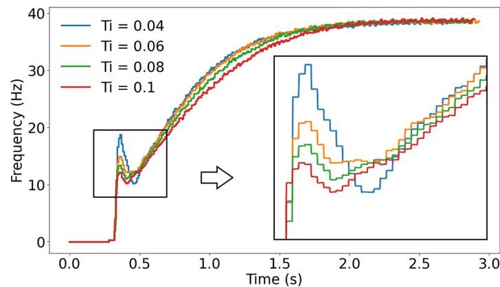
**Figure 22.** System frequency signal at the starting phase with  $K_p = 2$  and different  $T_i$ .
