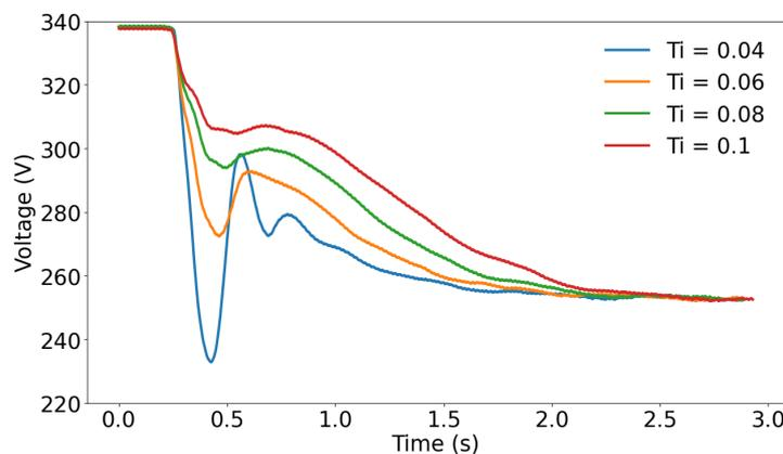
Figure 18. System voltage signal at the starting phase with  $K_p = 1$  and different  $T_i$ .
