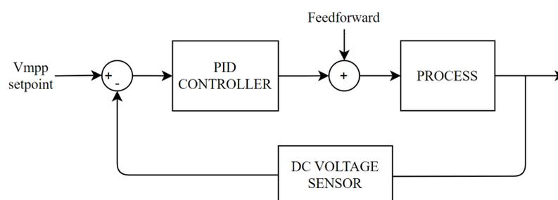
**Figure 4.** PID diagram with feedforward input.
