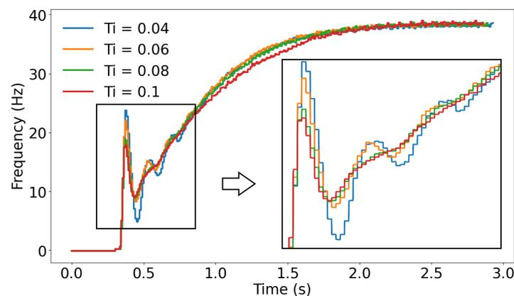
**Figure 23.** System frequency signal at the starting phase with  $K_p = 3$  and different  $T_i$ .
