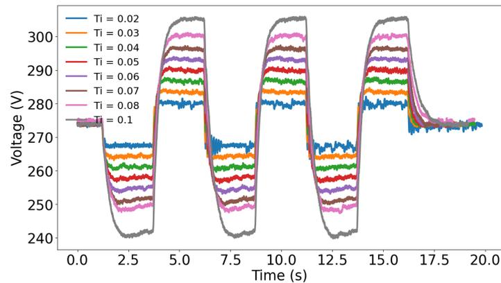
Figure 17. System voltage disturbance with a triangular feedforward signal, different  $T_i$  and  $K_p = 3$ .
