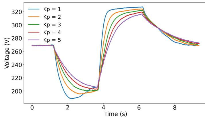
Figure 16. System voltage disturbance with a triangular feedforward signal, different  $K_p$  and  $T_i = 0.2$ .
