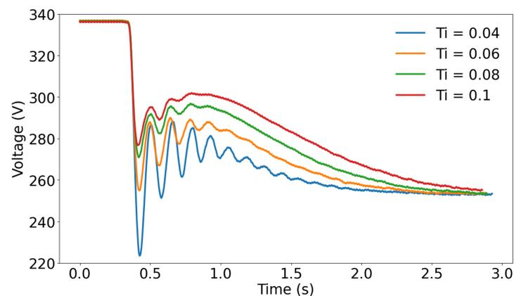
**Figure 20.** System voltage signal at the starting phase with  $K_p = 3$  and different  $T_i$ .
