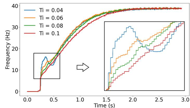
**Figure 21.** System frequency signal at the starting phase with  $K_p = 1$  and different  $T_i$ .
