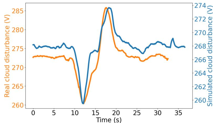
**Figure 14.** System voltage disturbance with real and simulated Cloud 2.
