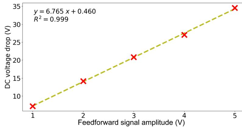
**Figure 9.** Relation between system voltage drop and feedforward signal amplitude for Cloud 1.
