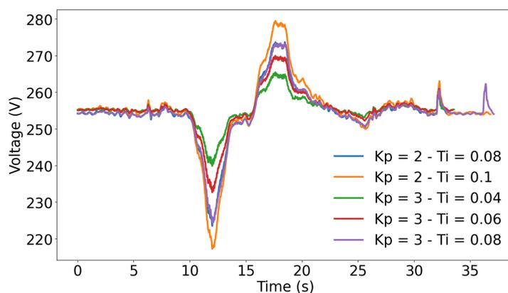
**Figure 24.** System voltage disturbance simulated for Cloud 2 with different PI constants.
