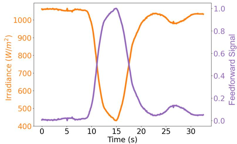
**Figure 7.** Feedforward signal, equivalent to the normalized and inverted irradiance, used to simulate the system voltage drop corresponding to Cloud 2.
