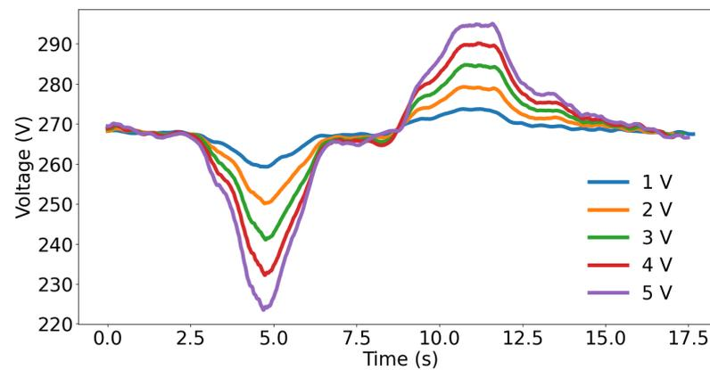
**Figure 12.** System voltage disturbances produced by different amplitudes of the feedforward signal for Cloud 2.
