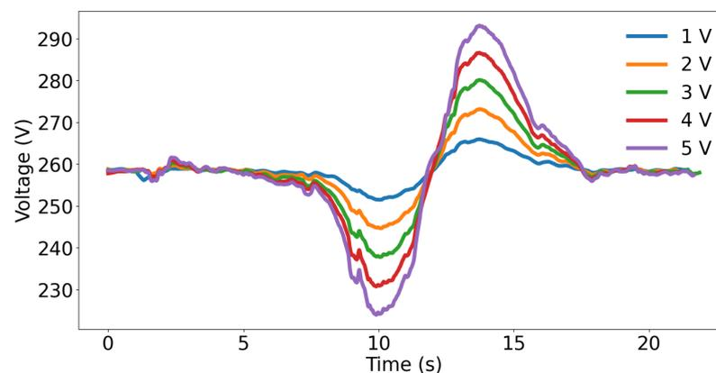
**Figure 11.** System voltage disturbances produced by different amplitudes of the feedforward signal for Cloud 1.
