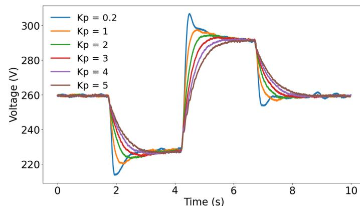
**Figure 15.** System voltage disturbance with a triangular feedforward signal, different  $K_p$  and  $T_i = 0.1$ .
