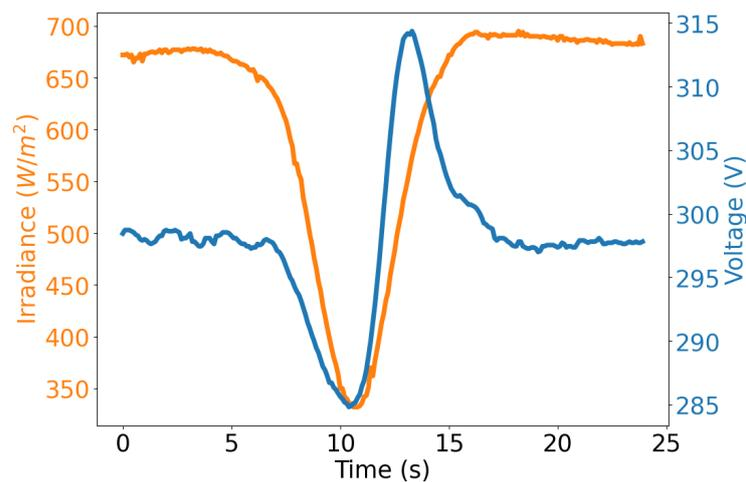
**Figure 2.** Cloud 1 (50.59% irradiance drop): irradiance fluctuation and corresponding system voltage disturbance.
