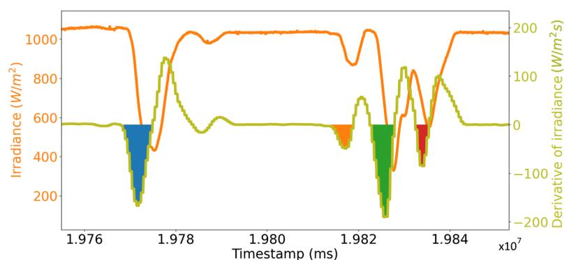
**Figure 1.** Cloud detection algorithm.
