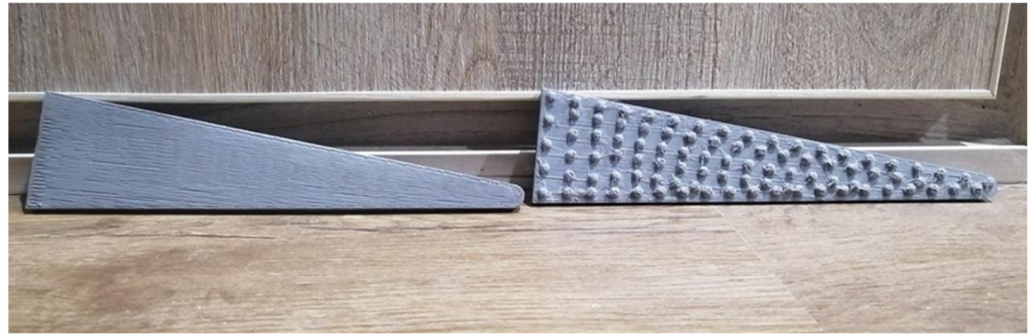
Figure 4. Prototypes of a normal and dimpled section of a turbine blade.
