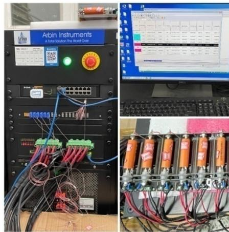
Figure 2. Arbin BT-ML-30V/10A battery tester.
